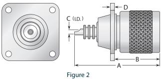
Figure 2 (Panel plug receptacle)
