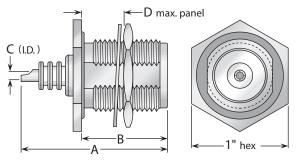
Figure 3 (Bulkhead jack receptacle)
