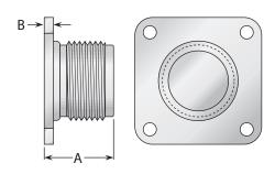
Figure 4 (Dummy receptacle)
