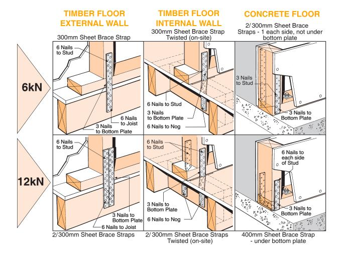
LUMBERLOK Sheet Brace Straps are available in 200, 300, 400 and 600mm lengths.
