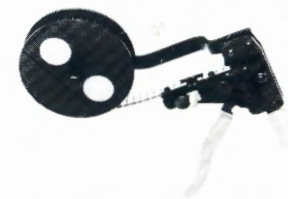
Hand Tool Part No. 169424-1 provided with reel-feeding device
