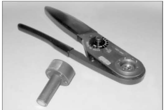
Crimp tooling M317 and locator VGE1 0078A
