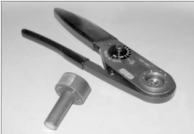
Crimp tooling M317 and locator VGE1 0077A
