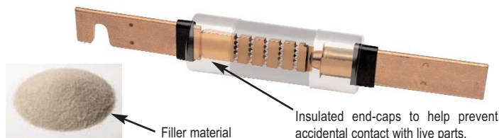
Figure 6. This is the LPS-RK100SP, a 100A, 600V Low-Peak, Class RK1, dual-element fuse that has excellent time-delay, excellent current-limitation and a 300,000A interrupting rating. Artistic liberty is taken to illustrate the internal portion of this fuse. The real fuse has a non-transparent tube and special small granular, arc-quenching material completely filling the internal space.
