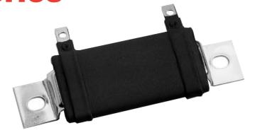
The FRW Series is designed for vertical or horizontal mounting, either singly or in stacks. Non-magnetic mounting brackets extending through the resistor allow easy and economical mounting. They also aid in heat distribution along its entire length and serve as conductors to transfer internal heat to the chassis.
