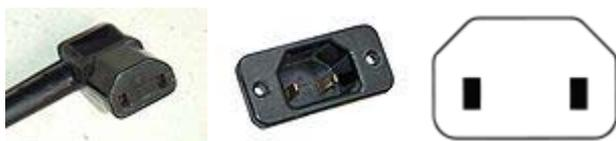
Similar to C13/C14 coupler, but unearthed. A C18 inlet will accept a C13 connector but a C14 inlet will not accept a C17 connector.
