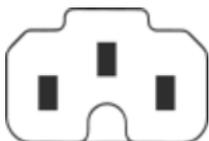
There is also a C15A/C16A coupler, with an even higher (155 °C) temperature rating.
