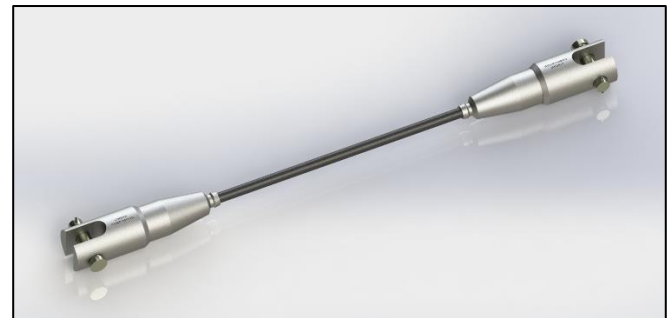
Figure 3 ~ Terminated Parafil® rope sample used for tensile testing.
