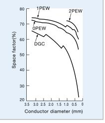
Figure 1: Comparison of magnet wire space factor
