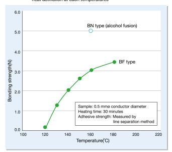
• Figure 11: Bonding characteristics of self-bonding wire in high temperatures
