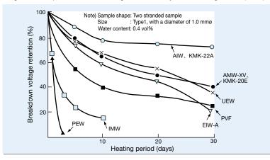
Table 4: Example of charge water resistance (Type1, with a diameter of 1.0 mm)
