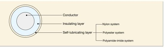
Table 6: Example: Applications of self-lubricating enamelled wire
