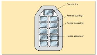
Figure 15: Appearance of Transposed wire
