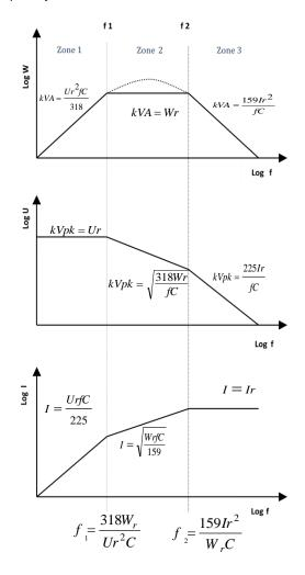
At frequencies below  $f_1(Zone1)$  the capacitor can be operated at it's maximum ac rating  $U_{\rm r}$
