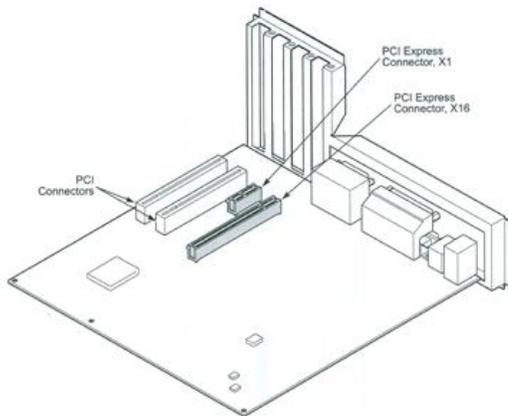
3. Remove the cover screw from the empty PCI slot's cover, set the screw aside.
