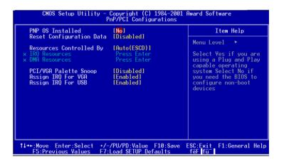
Figure 3-8: PnP/PCI configurations screen
