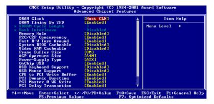
Figure 3-4: Advanced chipset features screen
