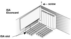
Figure 2. Inserting the Eiconcard S5x.
