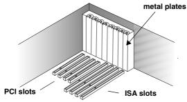
Figure 1. Locating a PCI slot
