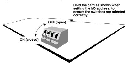
Figure 12. I/O Address Switch
