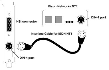
Figure 3. Connecting to the Eicon Networks NT1
