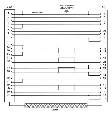
Figure 11. HSI Null-Modem Conversion Cable (300-033)
