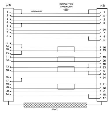
Figure 8. HSI V.24/V.35 Null-Modem Cable (300-031)
