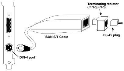
Figure 4. Connecting the ISDN S/T Cable
