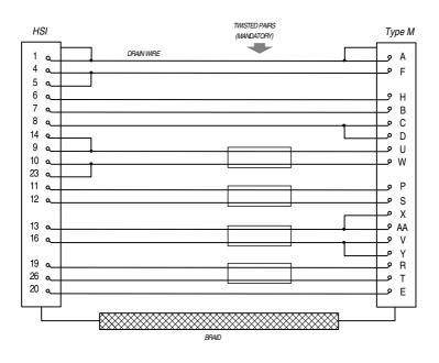
Figure 10. HSI V.35 Null-Modem Cable for AS/400 (300-047)
