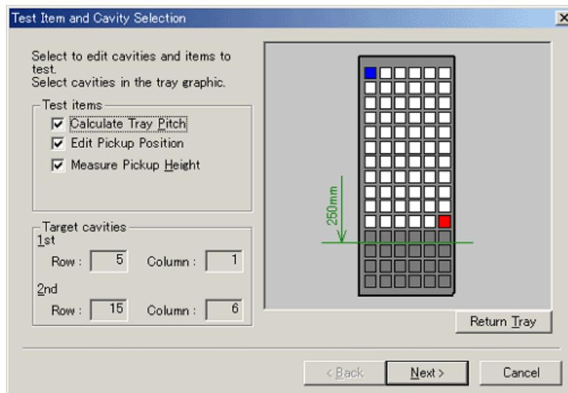
9. Select the type of tests which are to be performed in the dialog box that is displayed. If the [Calculate Tray Pitch] or [Edit Pickup Position] options are selected, proceed to the next step. If the [Measure Pickup Height] option only is selected, then go to step 18.
