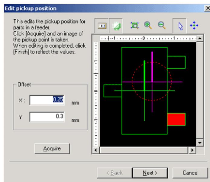
11. Check the pickup position in the X- and Y-direction using the displayed image. To move the pickup position, click the positioning button (the button with the four arrows) and then click in the image where the pickup should be performed.
