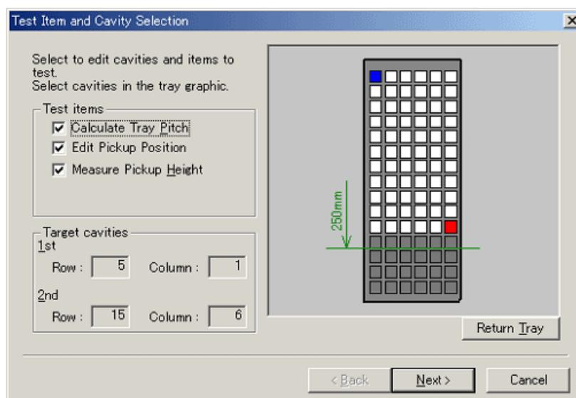
10. If the [Calculate Tray Pitch] option is selected, then specify two possible pick positions in the tray. If the [Edit Pickup Position] is only selected, then select only one pickup position. [Next] is not available until the required positions have been selected.
