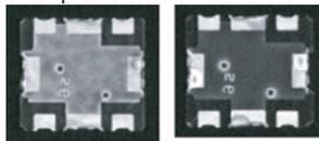
For these type of parts, the white area of the image can be different depending on the lot. Therefore, the surface of the part may appear bright or dark in the image. In order to be able to correctly vision process in both cases, it is necessary to define three leads (the right top, left bottom and right bottom leads).
