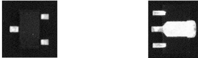
The defined lead area and actual captured image is substantially different, distinguish by the rectangular and non-rectangular lead shapes
