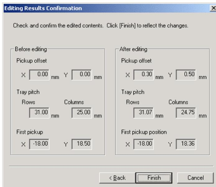
24. The offset and pitch results for the pickup position test are displayed. Check the results and if the results are acceptable, click [Finish]. It is possible to click [Back] to return to previous steps of the pickup test.
