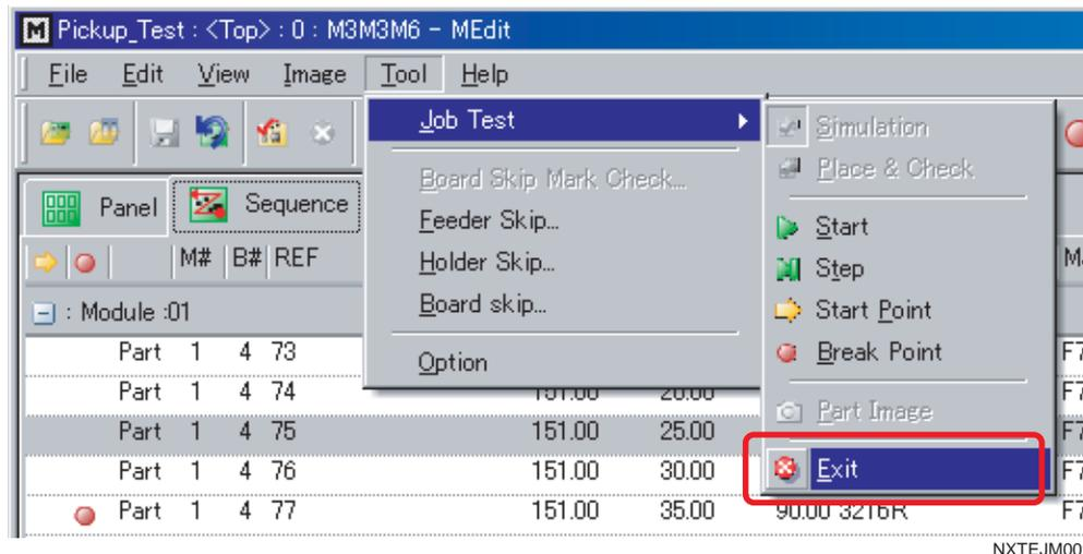
17. Once all testing for simulation mode has been completed, select [Job Test] - [Exit] from the [Tool] menu.
