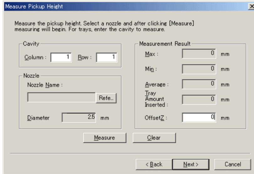
13. The [Measure Pickup Height] step is displayed. Ensure that the part has been advanced to the proper position (refer to section "6.6.4 Feeder index count and tape return method for pickup tests") then click [Ref.] to specify which nozzle to use for the test.
