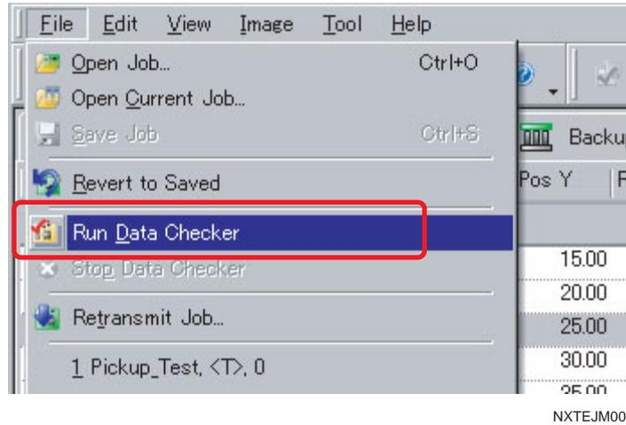
14. Once the sequences have been checked, click [Run Data Checker] from the [File] menu to check the job for any problems. Once the data checker has completed checking the job, retransmit the data back to the module.
