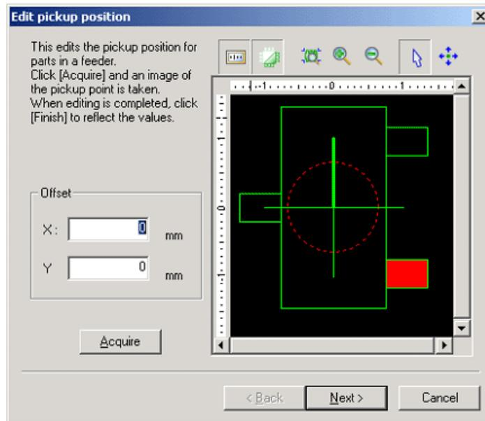
10. The [Edit pickup position] step is displayed. Ensure that the part has been advanced to the proper position (refer to section "6.6.4 Feeder index count and tape return method for pickup tests") then click [Acquire] to take a picture of the part in the feeder. A picture of the part is taken and displayed.
