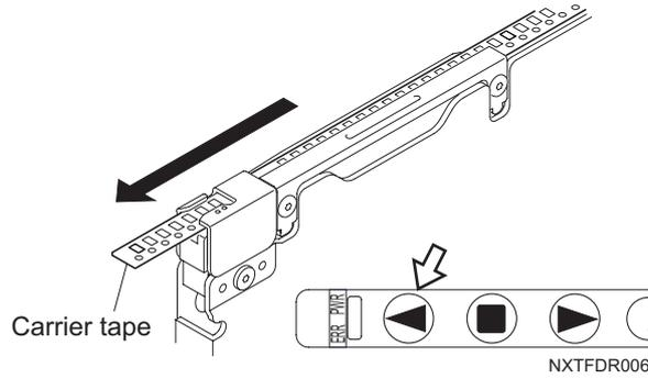
1. Check the chart and push the index button the number of times required to index the part forward.
