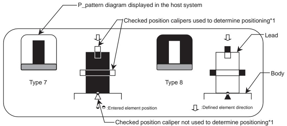
\*1 The caliper is a vision processing tool used for detecting the boundary between light and dark.
