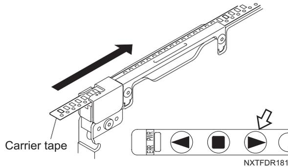
1. Check the part and index the part back the number of times it was indexed forward by pushing the back button the same number of times.
