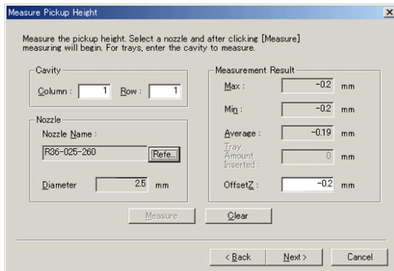
16. The results of the test are displayed and the Z offset is automatically determined. It is possible to manually edit this value.
