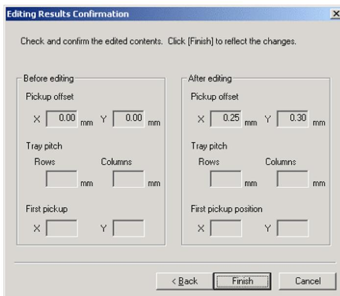
18. The offset results for the pickup position test are displayed. Check the results and if the results are acceptable, click [Finish]. It is possible to click [Back] to return to previous steps of the pickup test.
