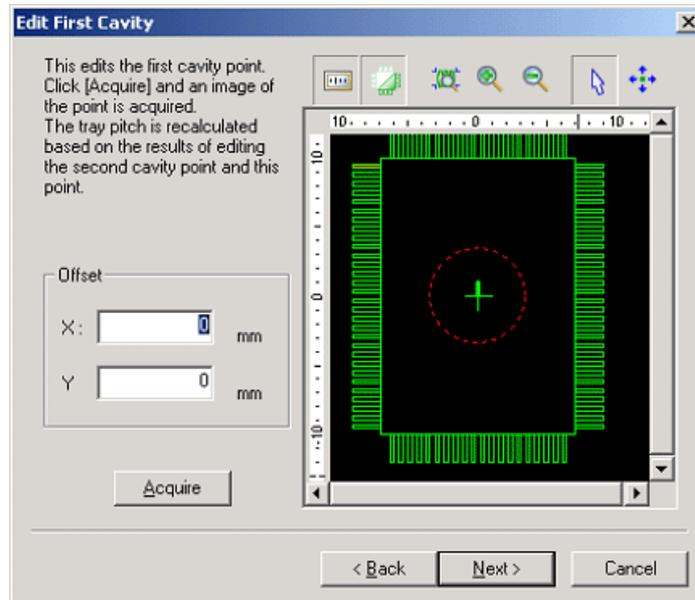
13. Check the pickup position in the X- and Y-direction using the displayed image. If the pickup position needs to be moved, click the positioning button (the button with the four arrows) and then click in the image of the graphic at which the pickup should be performed (the [Offset] values are automatically changed).
