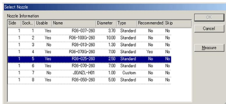
14. Select the nozzle to be used for the measurement in the dialog box that is displayed and then click [OK].
