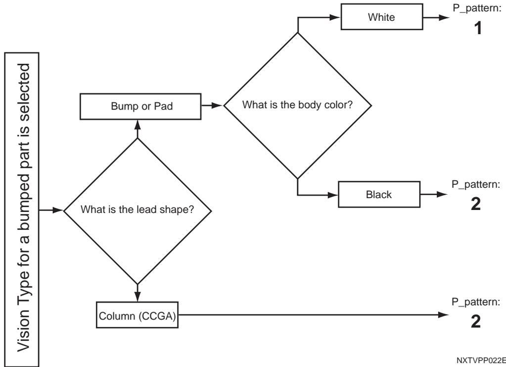
For backlight ledged parts (not supported by the NXT)
