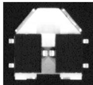
This part is like two three-pin minimolds facing each other in a white body.
