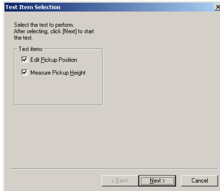
9. Select the type of tests which are to be performed in the dialog box that is displayed. If the [Edit Pickup Position] option is selected, proceed to the next step. If the [Measure Pickup Height] option only is selected, then proceed to step 13.
