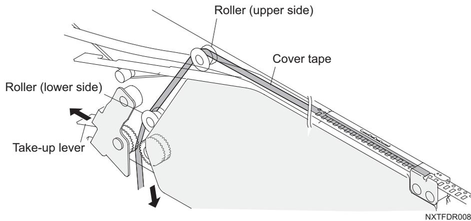
*Note: The take-up lever is designed to prevent looseness in the top film when rotated correctly (i.e., the tape is indexed forward). When rotated in the opposite direction, looseness in the top film develops. Eliminate this looseness manually by opening the take-up lever and gently pulling on the top film and then returning the take-up lever.*
