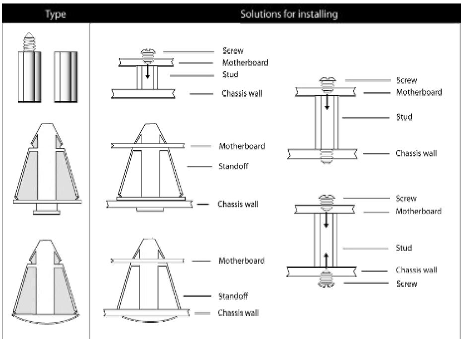
**TIP:** Use metal studs if possible, as they hold the motherboard into place more securely than plastic standoffs.
