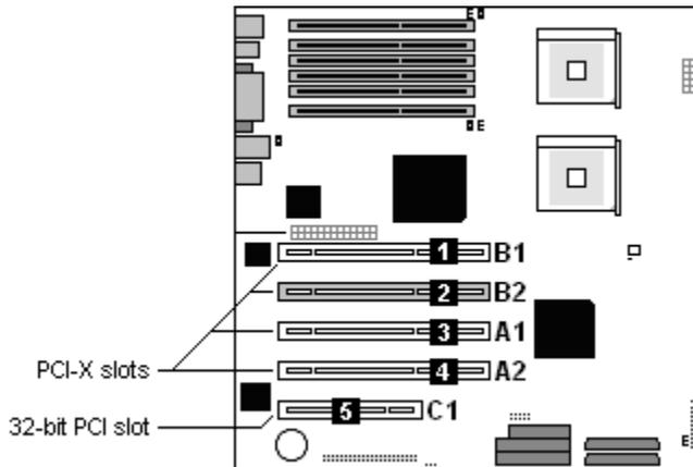
PCI slots A1, A2, B1 and B2 are all PCI-X slots while PCI slot C is a conventional 32-bit/33MHz PCI slot. However, PCI slots A1, A2, B1 and B2 will operate at the speed of the slowest PCI card that is installed into them. If a 33MHz PCI card is inserted into bus A, both A slots will operate at 33MHz. The same rule applies for Bus B slots. **A1 and A2 are BUS-A and B1 and B2 are BUS-B.**
