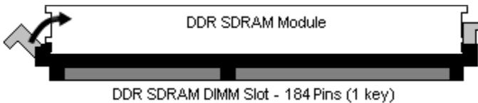
To remove the memory module, simply push the clamps outwards until the memory module pops up. Then, remove the module.
