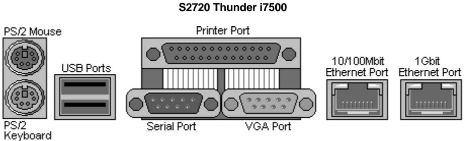
At times, the PS/2 ports for keyboard and mice may be mixed up. Simply remember that the port that is closest to the motherboard belongs to the keyboard and the one on top belongs to the mouse.
