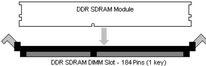
Once the memory modules are firmly seated in the socket, two clamps on either side will close and secure the module into the socket. Sometimes you may need to close the clamps yourself.
