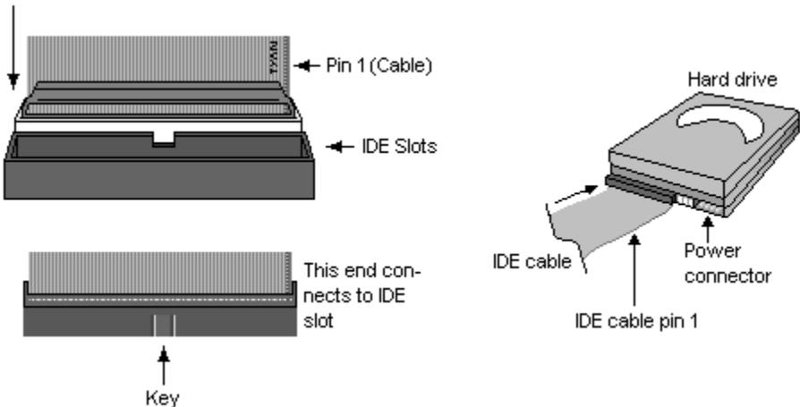
Simply plug in the BLUE END of the IDE cable into the motherboard IDE connector, and the other ends into the drive(s). Each standard IDE cable has three connectors, two being close to each other. The BLUE connector that is far on its own is the end that plugs into the motherboard whereas the other two connectors are used to connect to drives.
