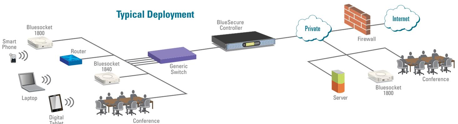
The BlueSecure Controller acts as a firewall between the wireless LAN access points and the wired LAN, and requires no changes to the existing wired LAN hardware or users' client software. Additional BlueSecure Controllers can be connected to provide seamless failover capability, as well as scalability and subnet mobility across the enterprise.
