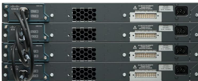
Figure 2. Cisco FlexStack Switch Stack
