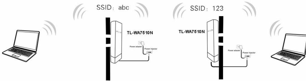
Figure 2-5 Hardware Installation of the TL-WA7510N in Standard AP -- Bridge mode
