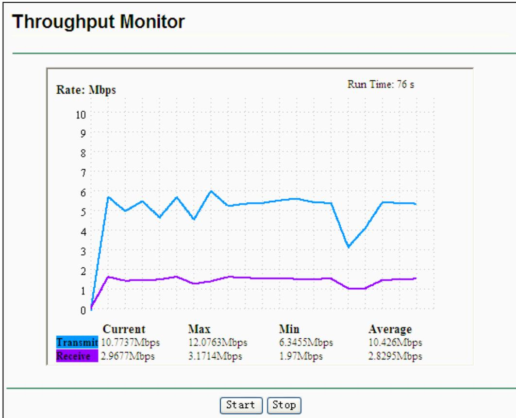
Figure 4-28 Throughput Monitor
