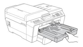
Pull out the paper support (1) until it clicks and unfold the paper support flap (2).
