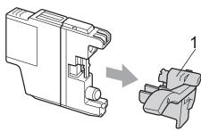
5 Each colour has its own correct position. Insert the ink cartridge in the direction of the arrow on the label.
