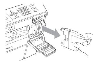
Open the new ink cartridge bag for the colour shown on the LCD, and then take out the ink cartridge.
