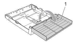
3 Using both hands, gently press and slide the paper length guide (1) and then the paper side guides (2) to fit the paper size.
