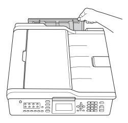
2 Slide the manual feed slot paper guides to fit the paper width that you are going to use.
