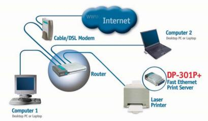
Next, make sure that the Printer is turned **OFF**. Connect the parrallel end of the DP-301P+ to the parallel port of the printer
