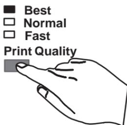
If you are using the AutoCAD or Windows drivers supplied with the plotter, the print quality setting (or an equivalent) within the driver will override the front-panel setting; *the front-panel light which is illuminated will change accordingly until this print job is finished.*
