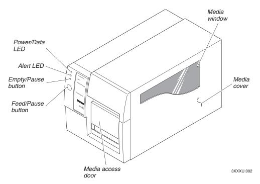
**Printer front view:** This illustration shows the features on the front of the printer.
