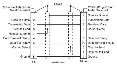
**RS-232 null modem cable for PC/AT:** This illustration shows the pin assignments for the RS-232 null modem cable for PC/AT (P/N 048693).
