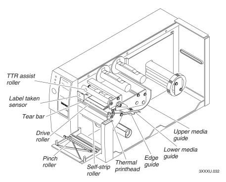
**Printer parts:** This illustration shows the printer parts that need to be cleaned. For a maintenance schedule of each part, see the Printer Maintenance Schedule table on pages 32-33.
