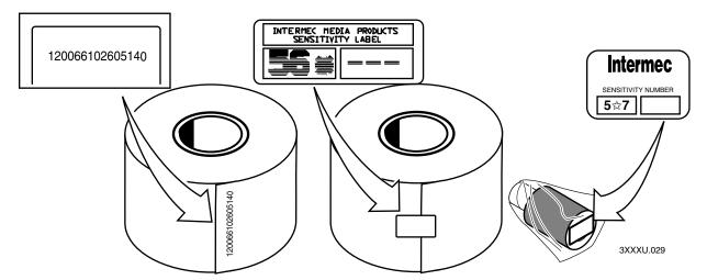
**Media sensitivity number:** This illustration shows you where to find the media sensitivity number. Note that some ribbon rolls have the media sensitivity number printed inside of the core.
