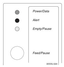
**Front panel:** This illustration shows the front panel LEDs and the Feed/Pause button.
