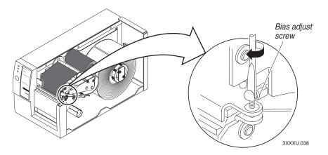
**2** To compensate for uneven print quality, turn the bias adjust screw as shown. Adjusting the bias adjust screw causes the printhead to rest evenly on the drive roller and results in even print quality.
