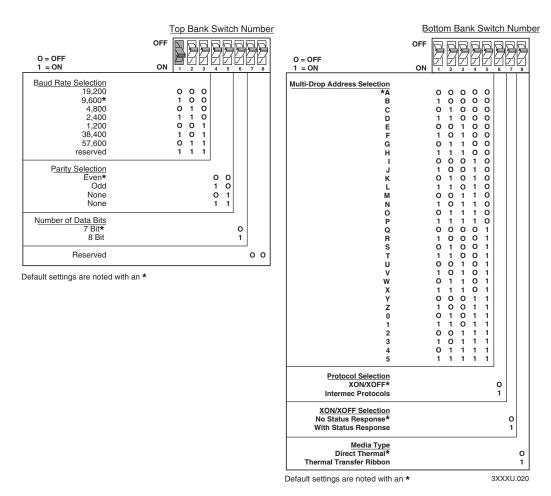
**DIP switch settings:** These charts illustrate the settings for the DIP switches on the top and bottom banks. For a description of each setting, see the DIP Switch Settings Descriptions table on page 12.
