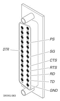
**Serial port pin assignments:** This illustration shows the serial port pin assignments.
