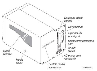
**Printer back view:** This illustration shows the features on the back of the printer.
