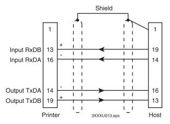
**RS-422 serial interface:** This illustration shows the pin assignments for the RS-422 serial interface. The host in this case includes Intermec products that support RS-422. Non-Intermec controllers may have different pin assignments.
