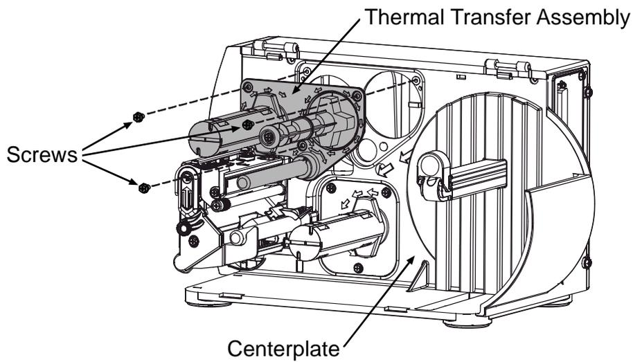
4. Remove the Screw and Washer securing the Supply Hub to the Thermal Transfer Assembly.
