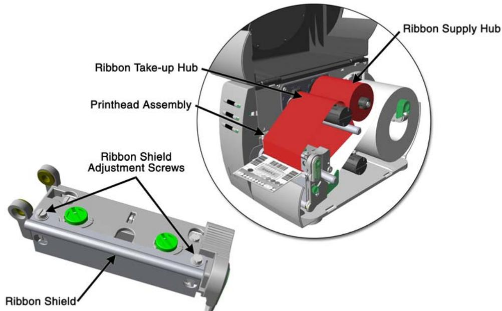
7. Install operating media and ribbon. Set the Media Width Adjustment, as needed (see Section 2.3). Send your label format to the printer from the host. Examine the printed labels; readjust the Ribbon Shield slightly, if needed.
