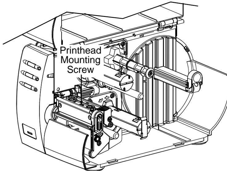
3. Unlatch the Printhead Assembly. While holding the Printhead, raise the assembly. Disconnect the two cables and then remove the old Printhead.
