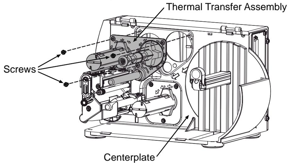
4. Remove the C-clip and Outer Bearing from the Thermal Transfer Assembly.
