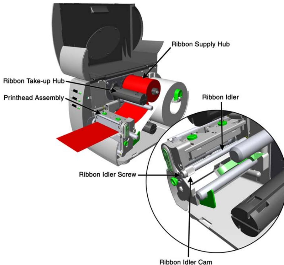
5. Attach the ribbon to the Ribbon Take-Up Hub then proceed according to printer type –
