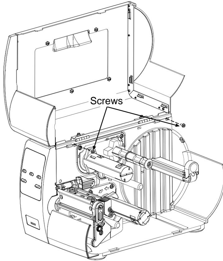
4. Lift the cover up and off the printer.
