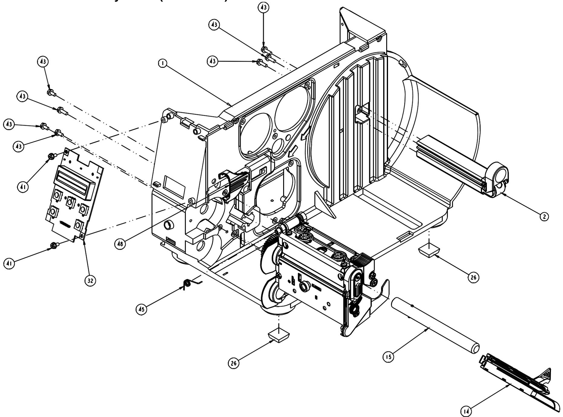
**D. Printer Assembly 2 of 3 (53-2153-03)**
