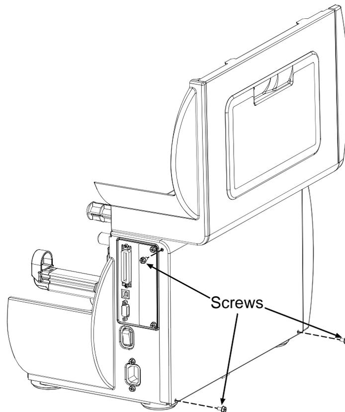
3. Open the cover and remove the two Screws from the inside of the printer, as shown.
