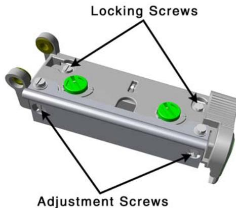
5. Turn each Adjustment Screw clockwise about a ¼ turn (or an 1/8 turn for finer adjustments, see note below). Print another test label and examine the print quality. Repeat this step until labels are produced with an even print contrast and an acceptable print quality.
