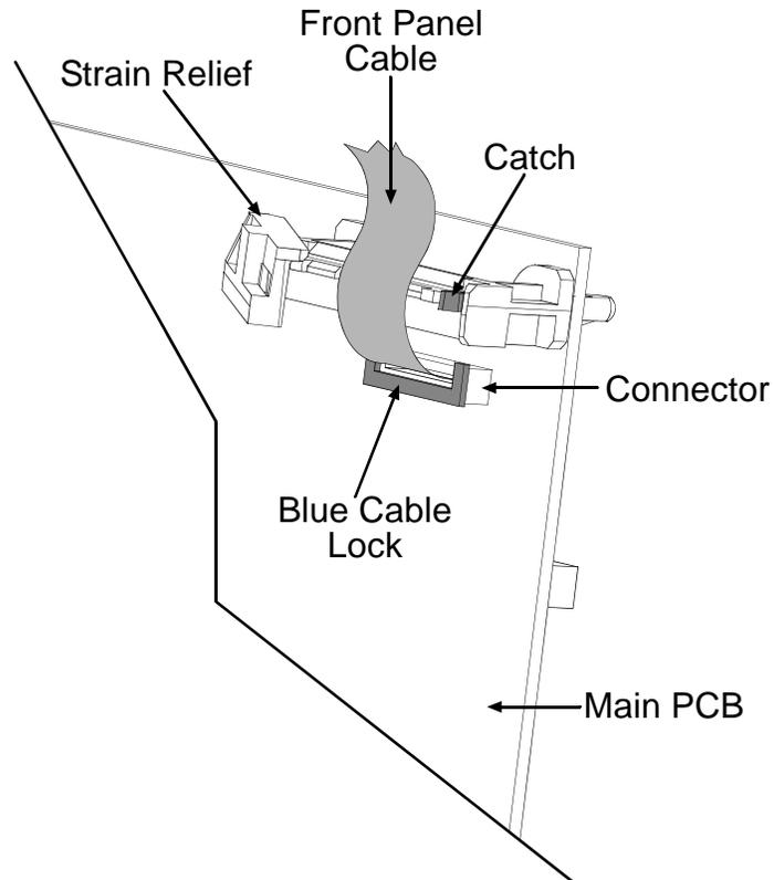
6. Remove the two Screws securing the Front Panel PCB to the printer (if you have a Display-Equipped Model, first remove the Bezel, as shown below). Move the Front Panel PCB away from the printer slightly, disconnect the Front Panel Cable, and then remove the Front Panel PCB.
