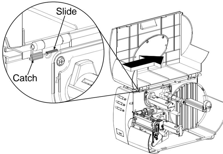
4. Lift the cover up and off the printer.
