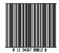
**Bar Code L:** Interleaved 2 of 5 w/modulo 10 checksum and shipping bearer bars
