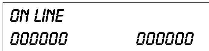
The LCD Panel will display the ON LINE status on the top line of the display and the bottom line will contain the label quantity status. The ON LINE message will be changed to OFF LINE whenever the printer is switched OFF LINE via the **START/STOP** key.
