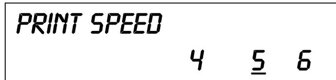
1. Use the START/STOP key to step the underline cursor to the desired speed setting.
