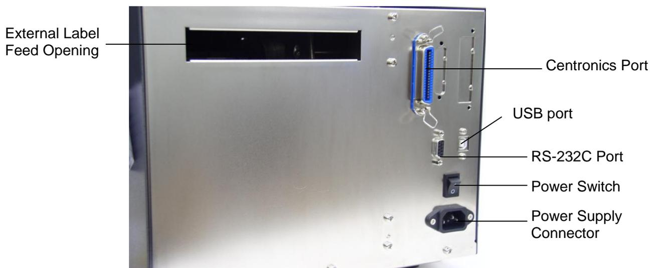
Figure 2. Printer rear view
