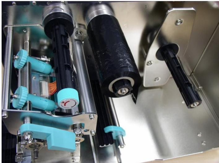
**Figure 5. Ribbon supply spindle installation**
