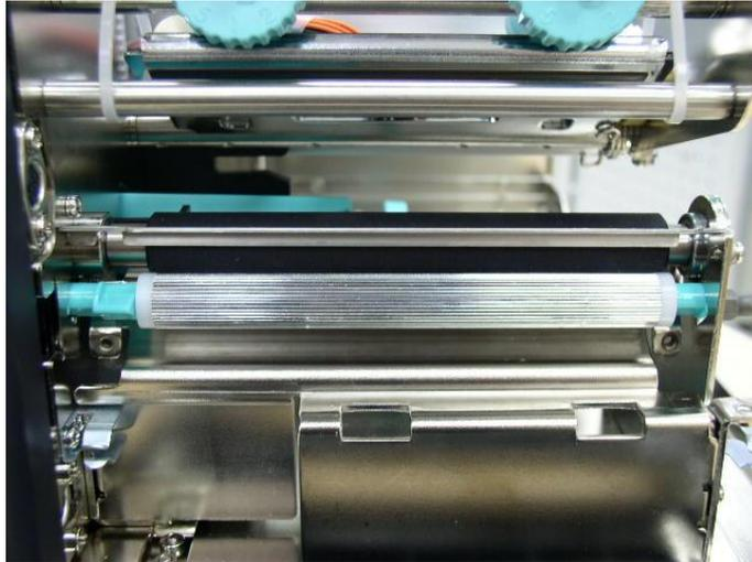
4. Fasten the leaf springs and washers with screws to fix the left and right side bush.
