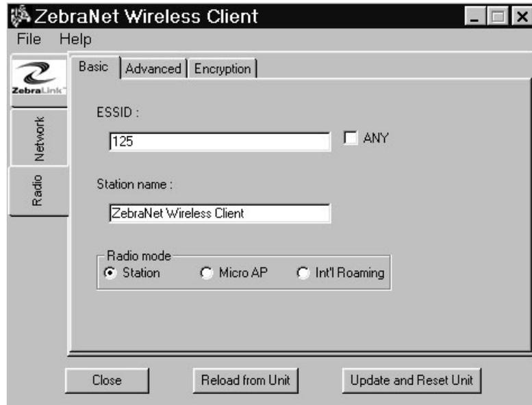
**Figure 6-28. The ZebraNet Wireless Client dialog with Radio>Basic tab open**
