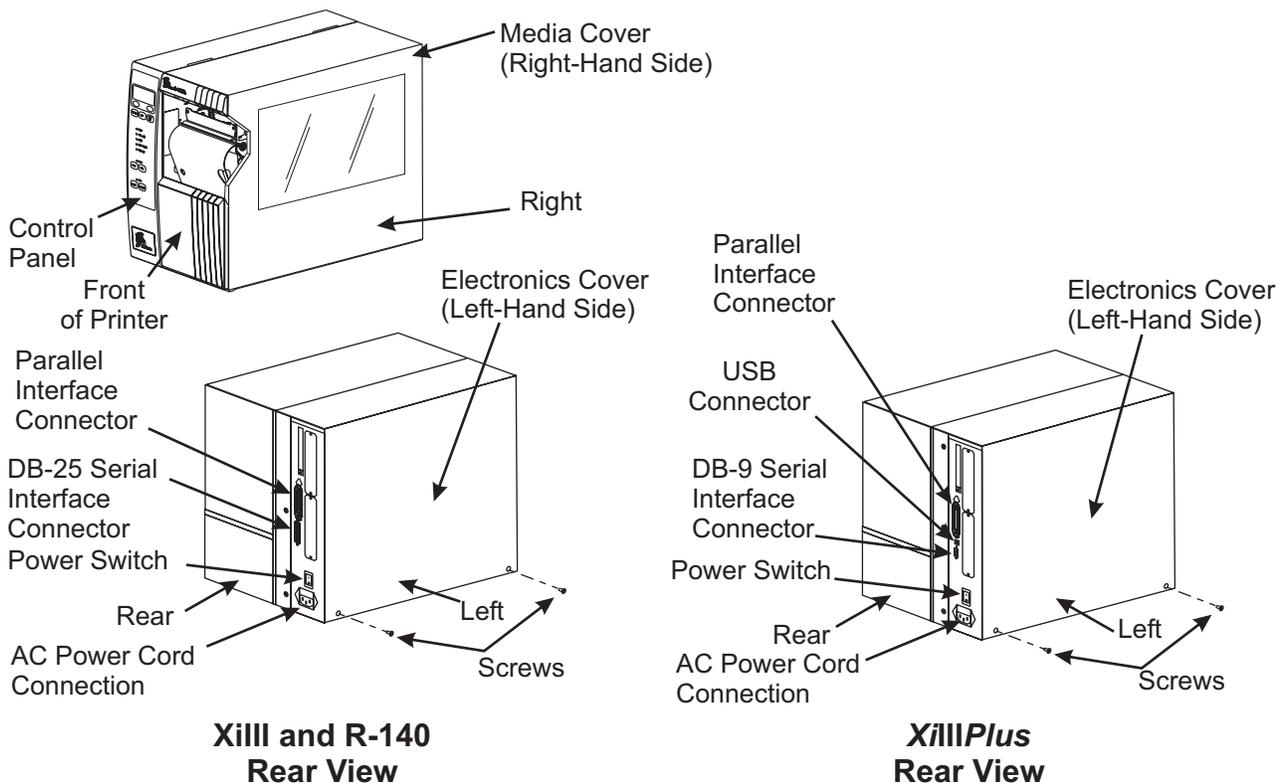
**Figure 4-4. External Printer Components Orientation**
