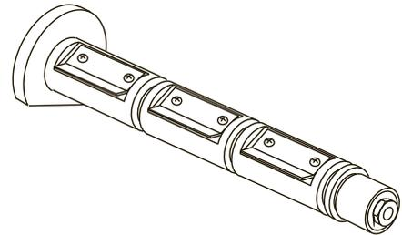
**NOTE: Ensure that the core is pushed up against the stop on the ribbon supply spindle and that the ribbon is aligned squarely with its core. If this is not done, the ribbon may not cover the printhead entirely on the inside, exposing print elements to potentially damaging contact with the media.**
