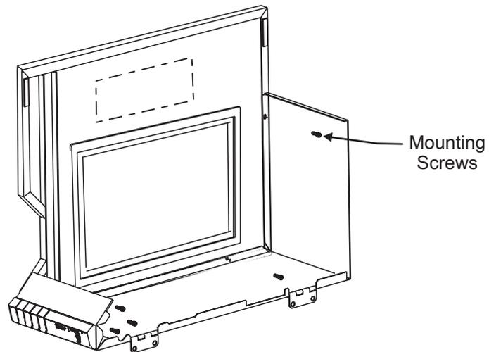
4. Install new door using the screws removed in step 2.
