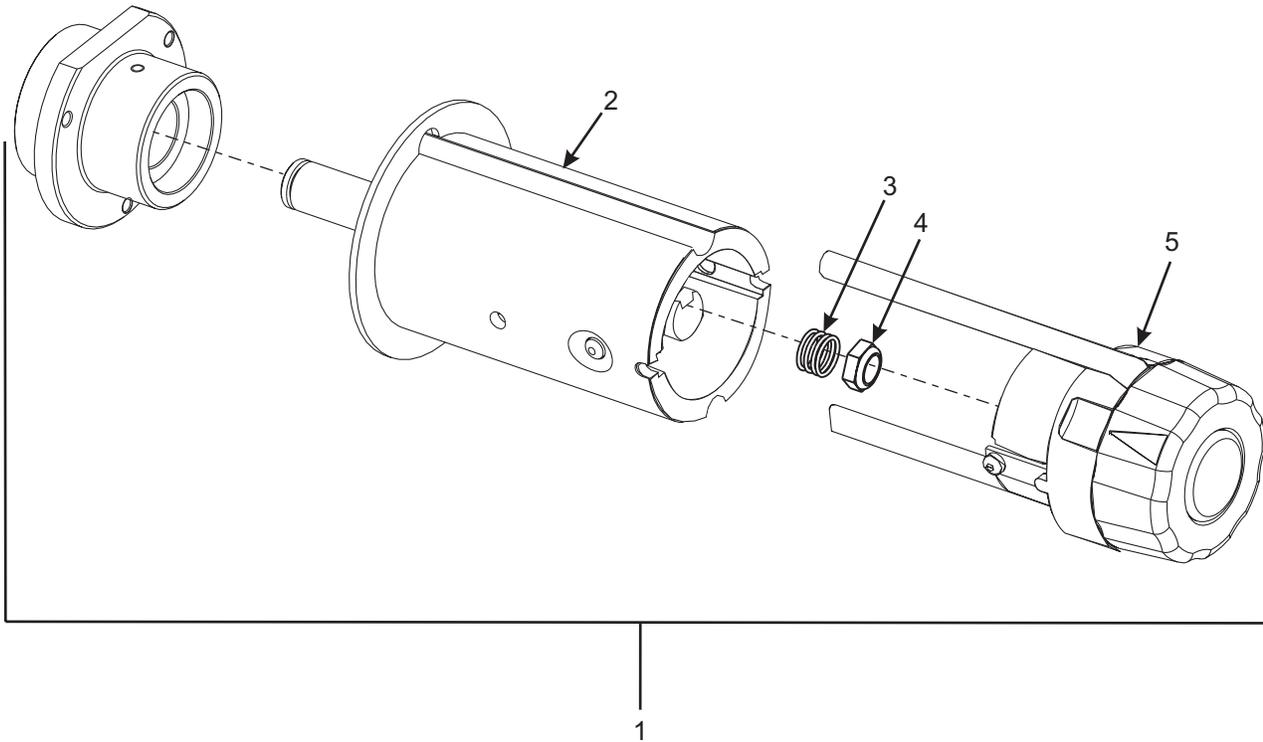
**Figure 5-16. Ribbon Take-Up Spindle Assembly**
