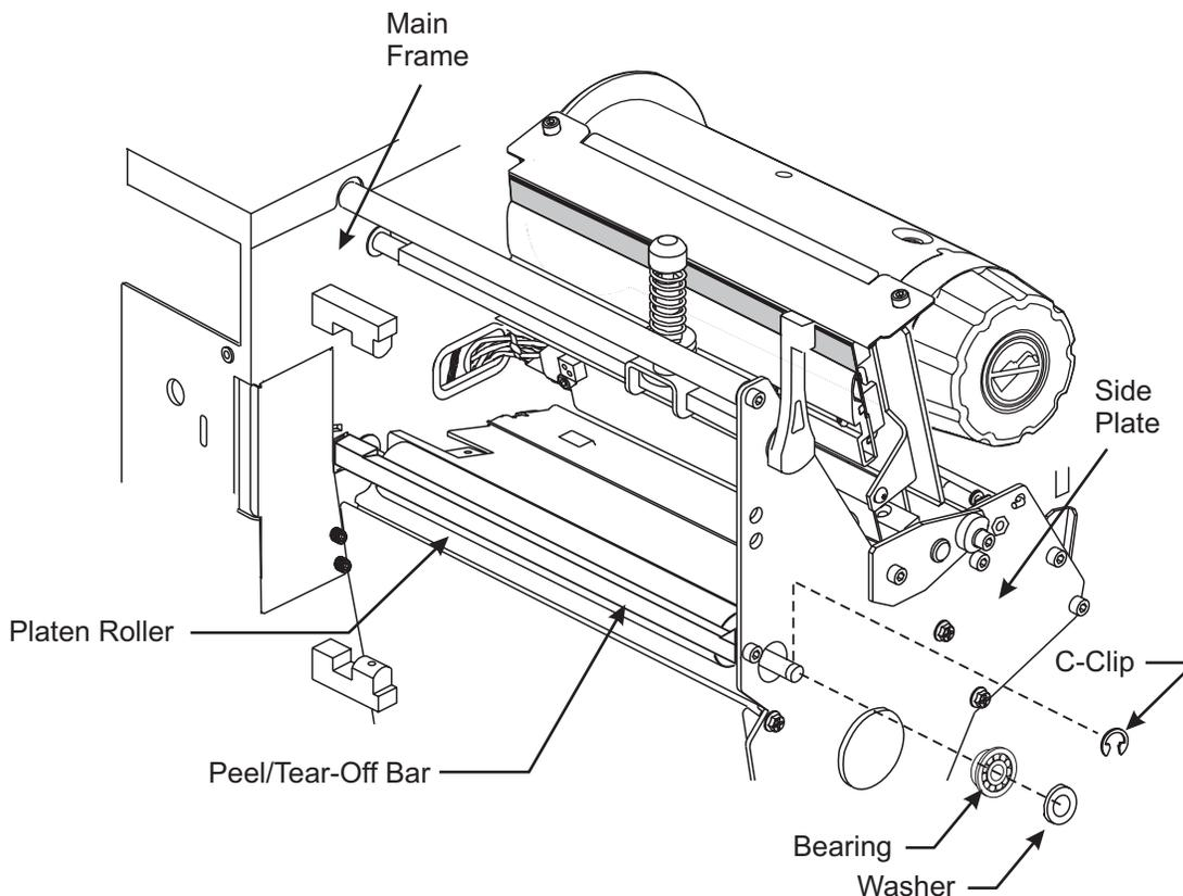
**Figure 4-56. Freeing Side Plate for Removal**
