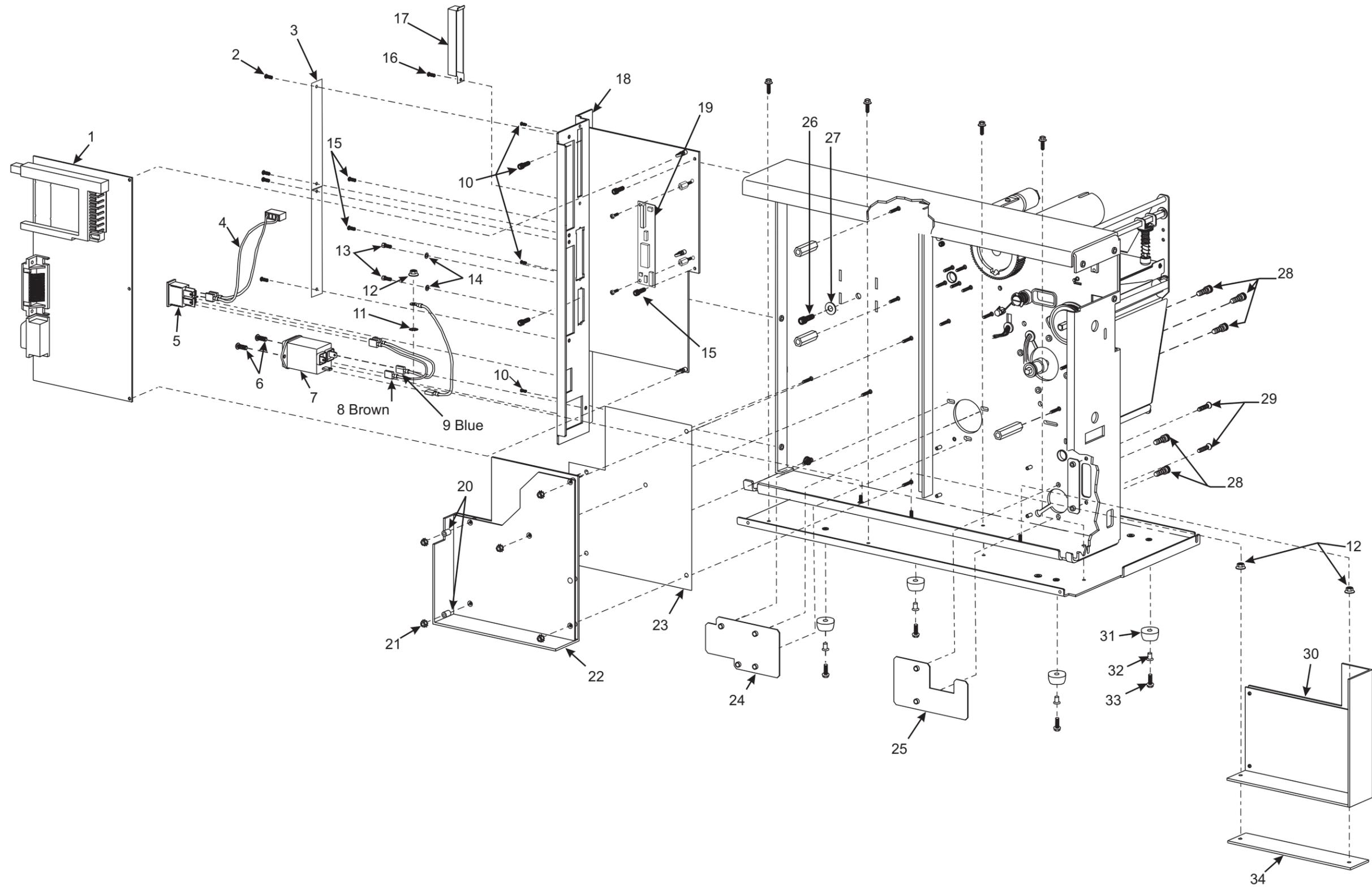
Figure 5-7. Print Mechanism X1111 Printers (View 3)
