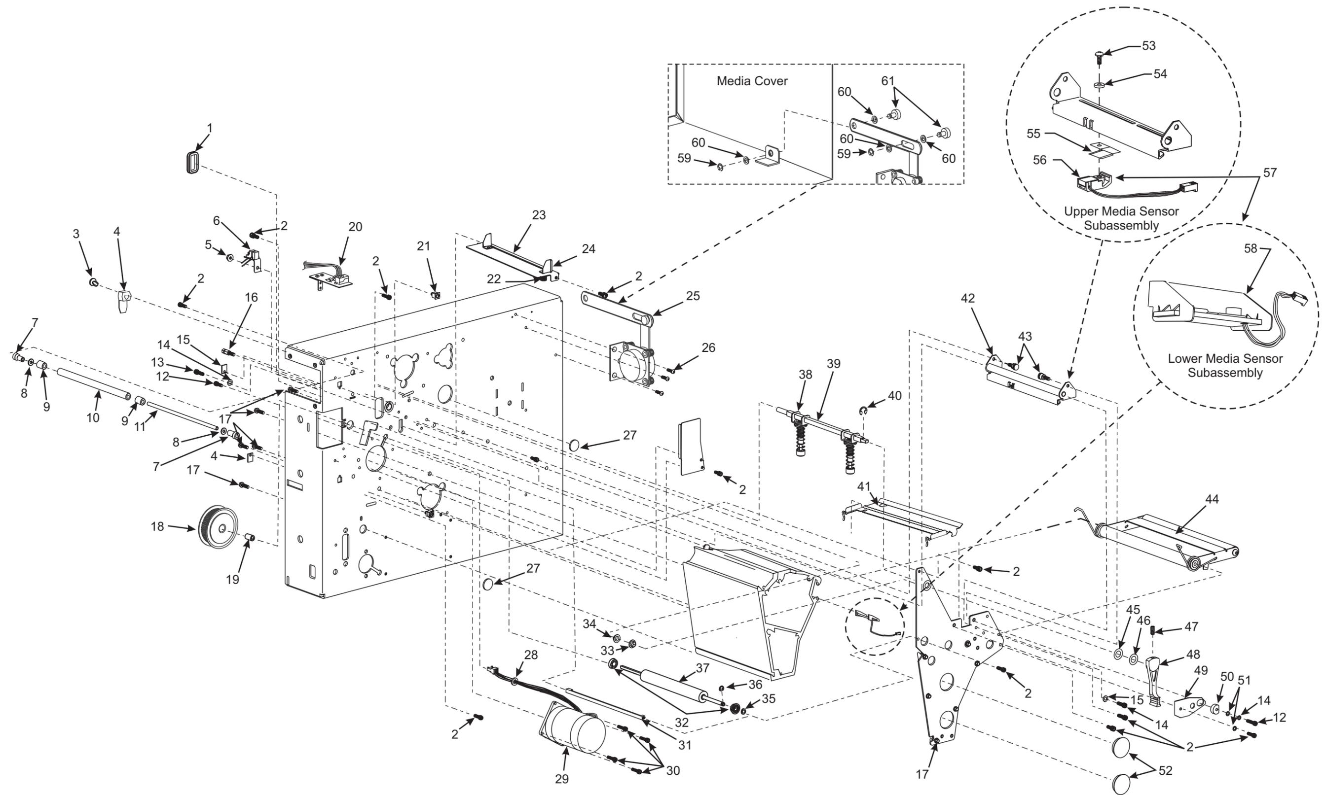
Figure 5-9. Print Mechanism 220XiIII (View 1)
