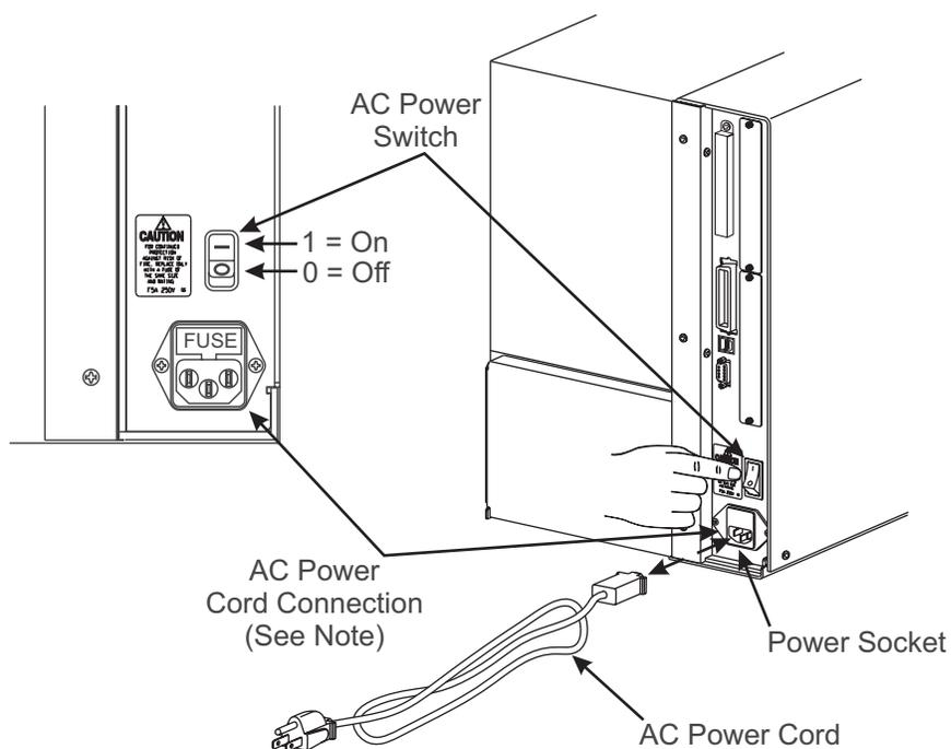
**NOTE:** Depending on configuration, the power entry module may not have a user-replaceable fuse.
