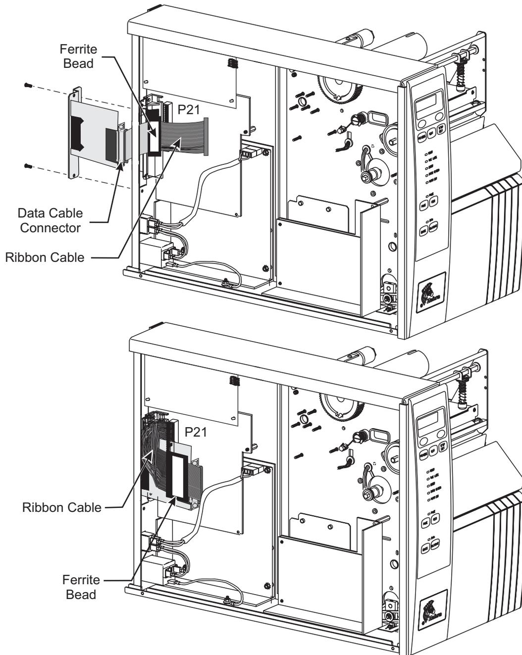
**Figure 6-18. XiiiPlus Internal PrintServer II Board Installation**
