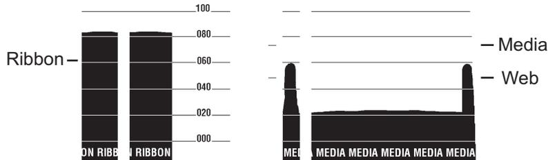
**Figure 2-16. Sensor Profile Sample Label**
