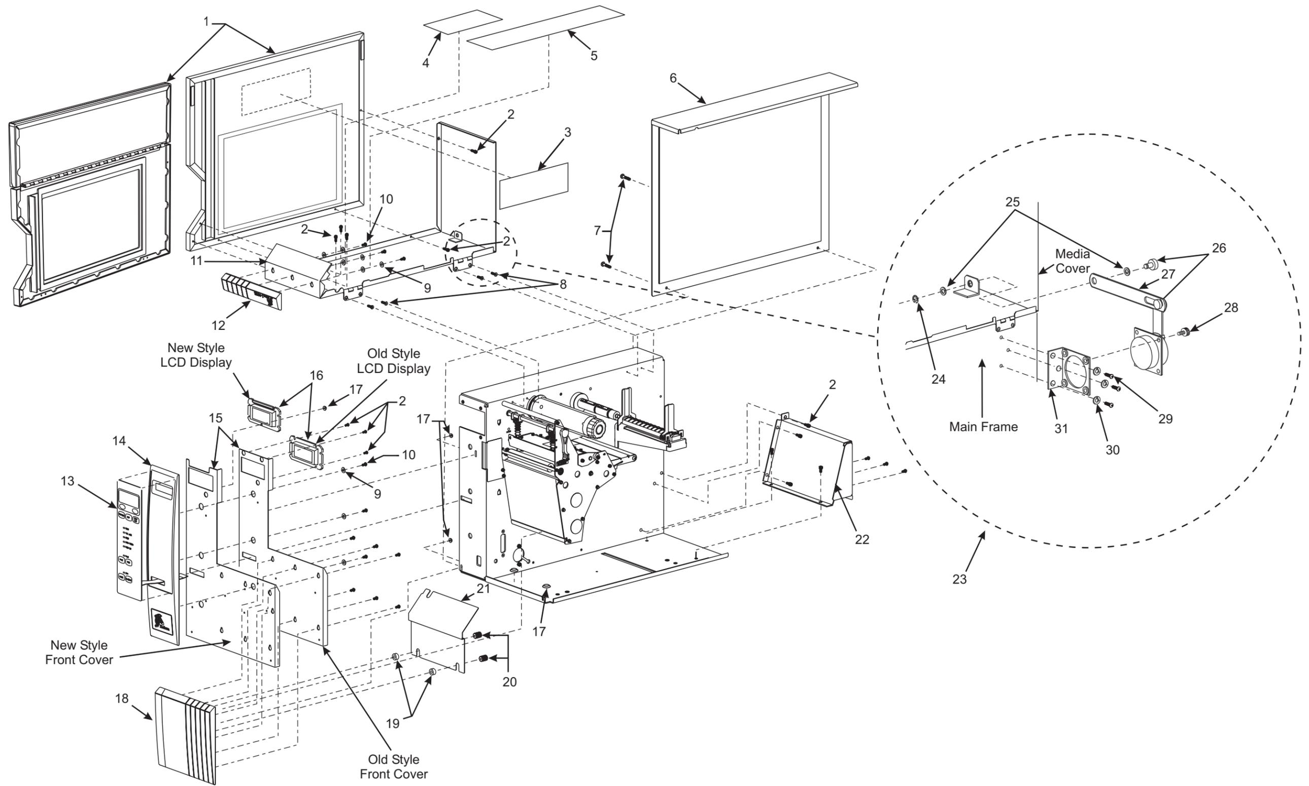
Figure 5-4. Final Assembly 220XiIII Mechanical
