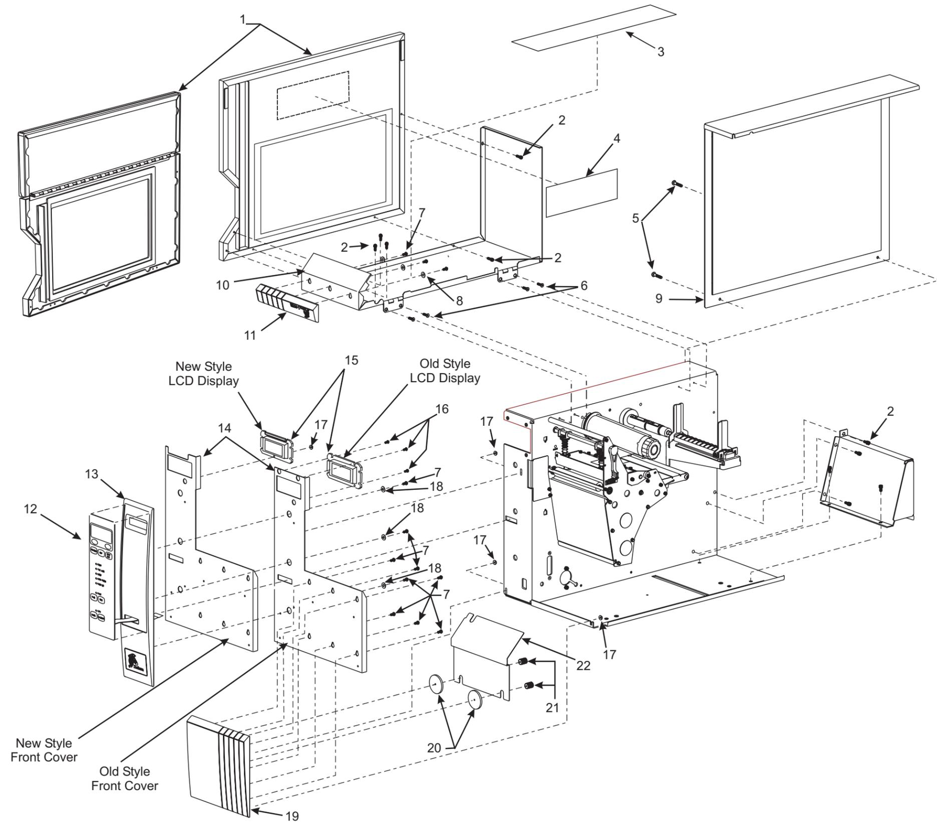
Figure 5-1. Final Assembly 90/96/140/170Xiii/XiiiPlus and R-140 Mechanical
