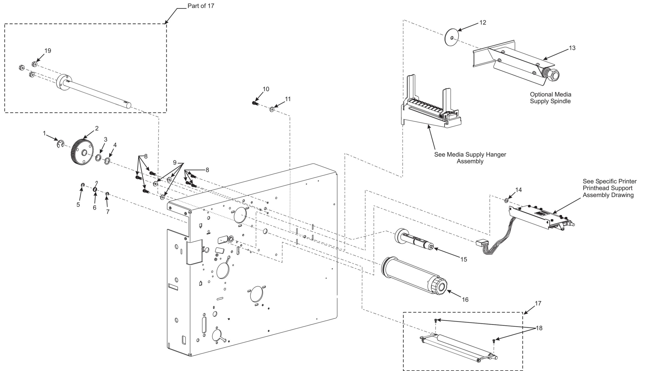
Figure 5-6. Print Mechanism for 90/96/140/170XiIII/XiIIIPlus and R140 (View 2)
