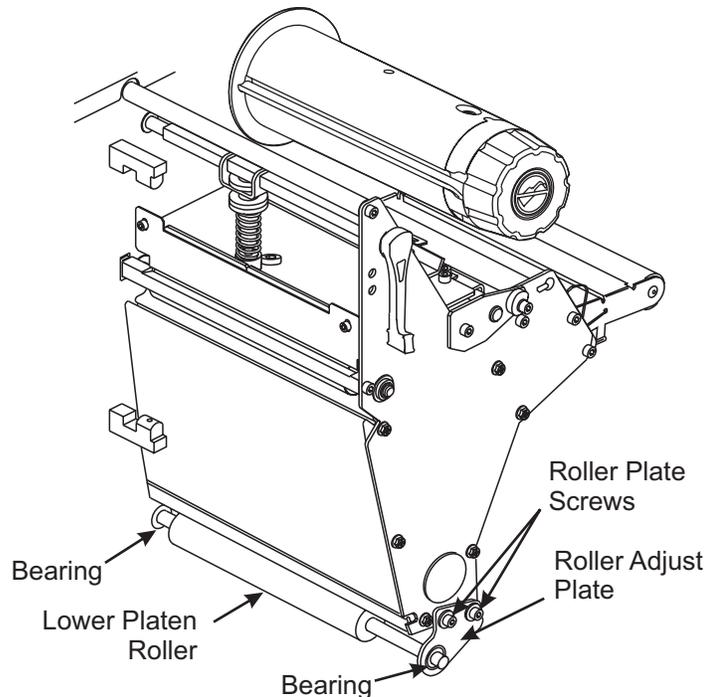
**Figure 4-28. Peel-Off Lower Roller Alignment**
