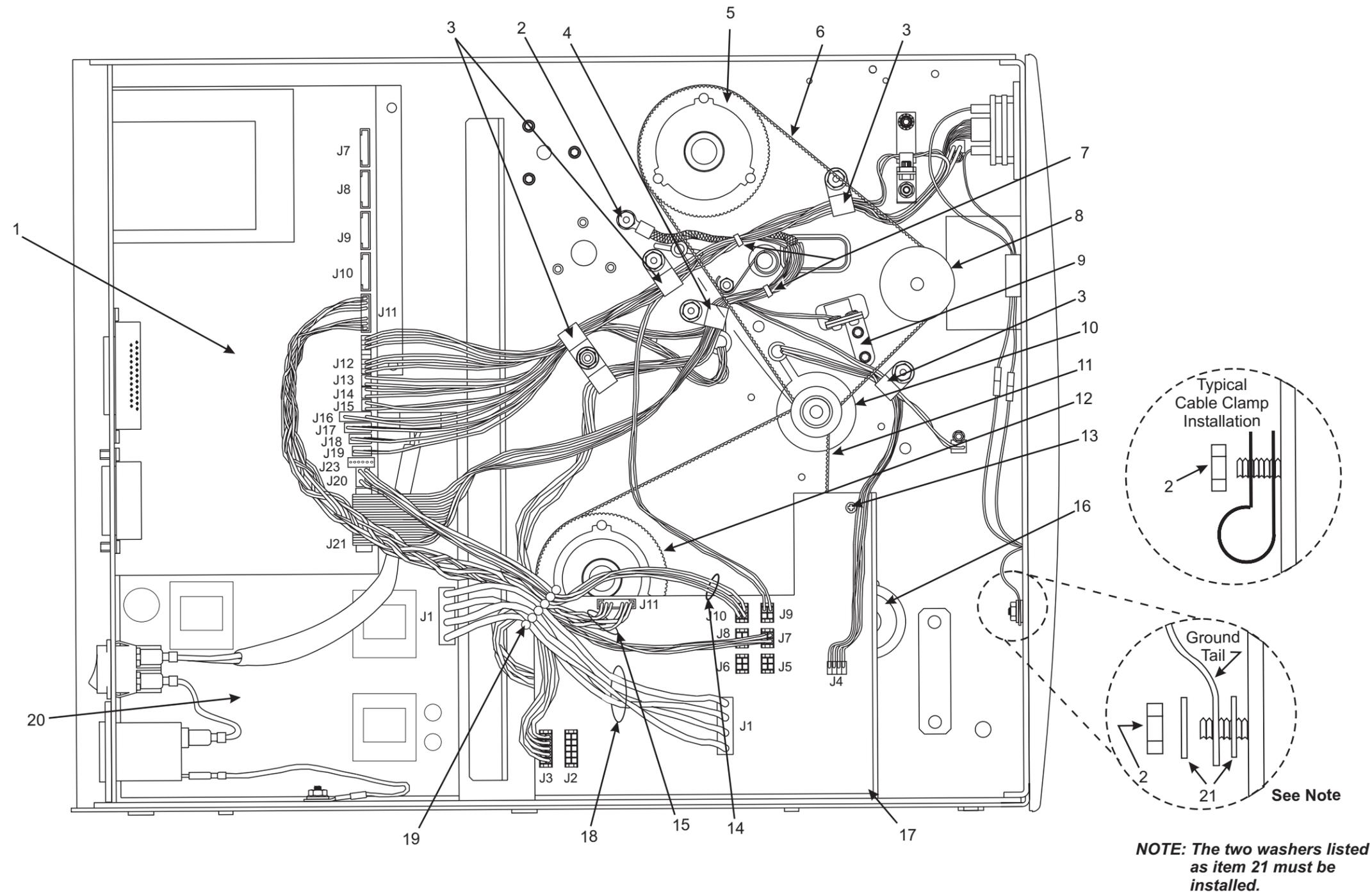
Figure 5-2. Final Assembly Electrical (X1111 and R-140)
