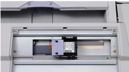
Note: Imprinter is the device for recognizing scanned documents by imprinting numbers on each document. fi-486PRFR enables users to store image data with imprint numbers on.
