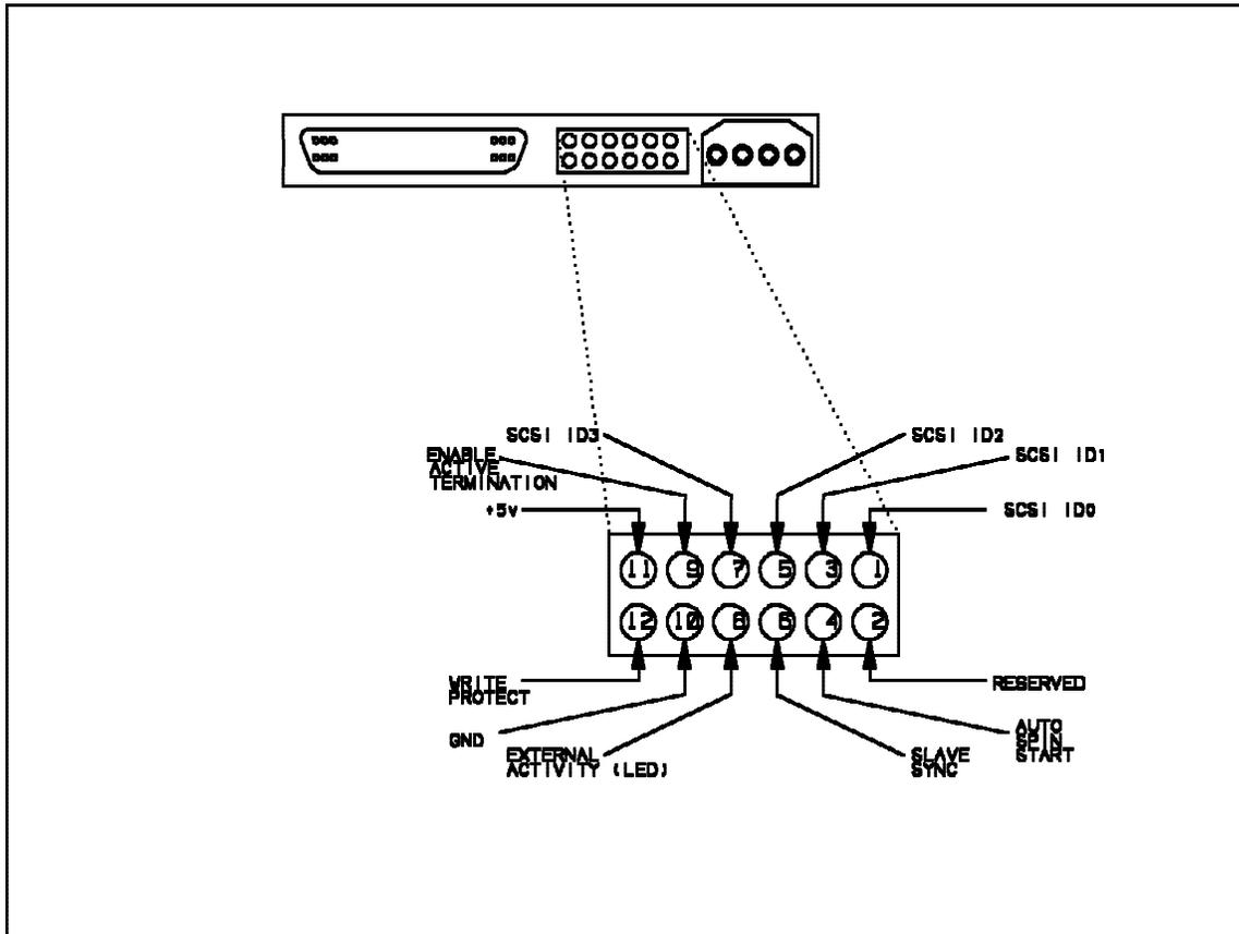
Figure 34. Auxiliary Connector on the 68 pin Connector
