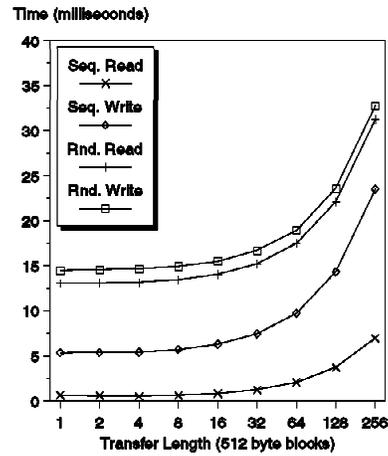
Figure 13. Read Caching enabled, Re-instruction Times = 50-150ms, no TCQing
