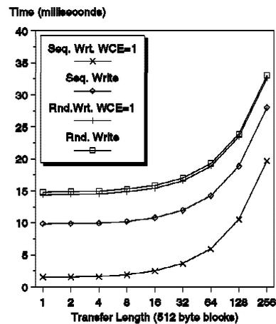
Figure 15. Read Caching enabled, Re-instruction Times = 0ms, no TCQing
