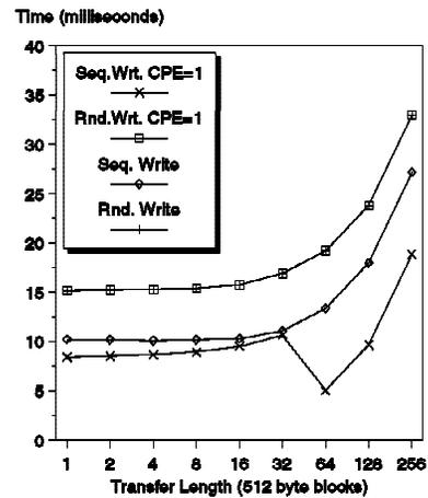
Figure 19. Read Caching & Concurrent Command Processing enabled, TCQing
