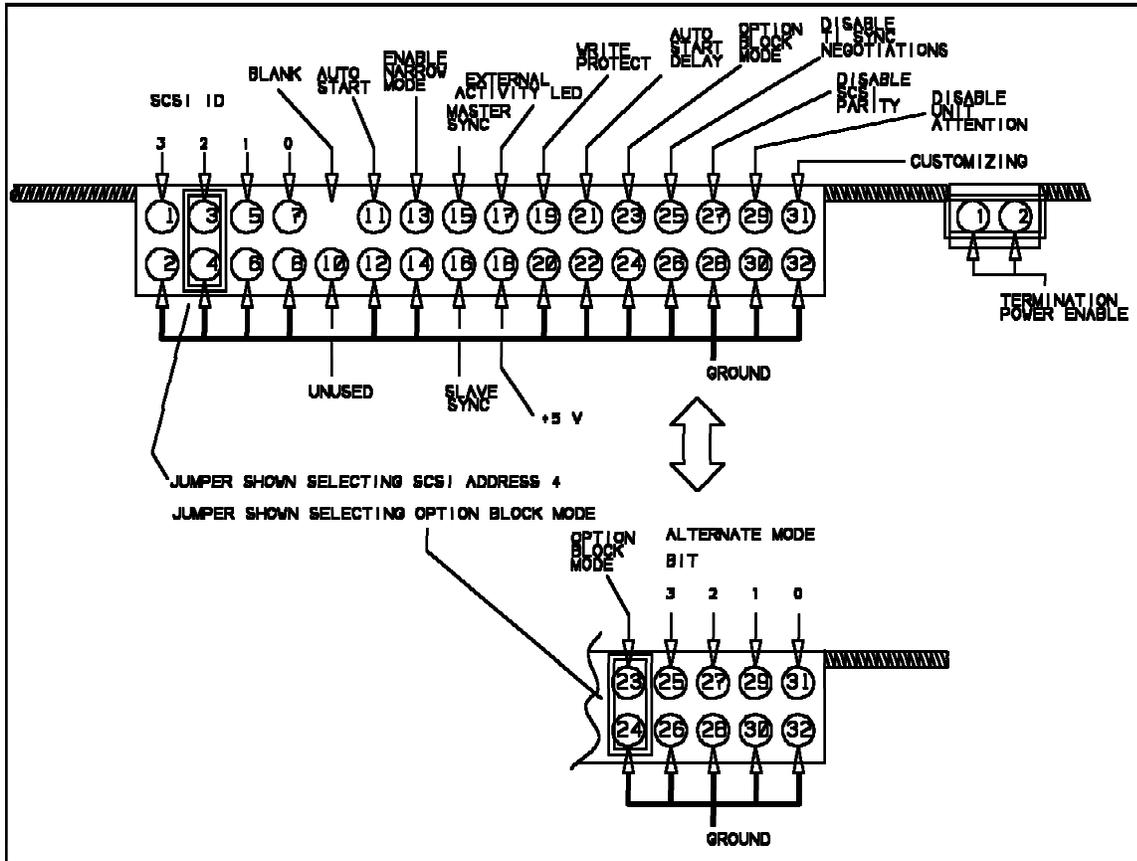
Figure 32. 68 pin Differential Front Option Jumper Block
