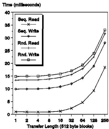
Figure 14. Read Caching enabled, Re-instruction Times = 0ms, no TCQing
