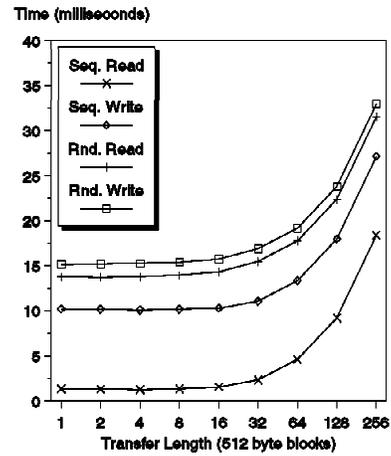
Figure 17. Read Caching enabled, TCQing used
