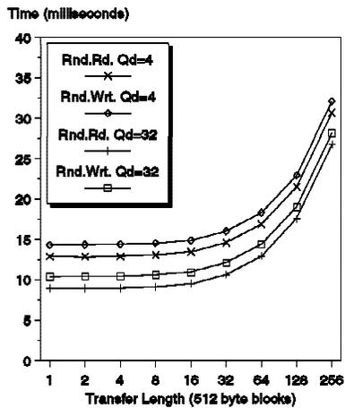
Figure 18. Read Caching & Unrestricted Command Reordering enabled, TCQing
