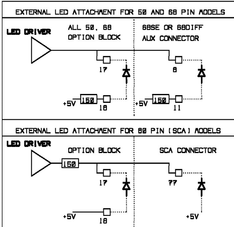
Figure 35. External LED Connections
