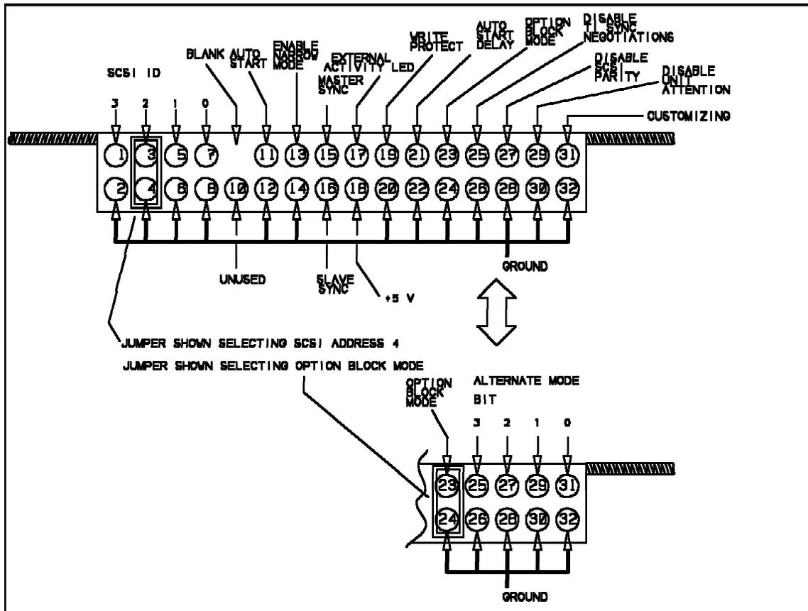
Figure 33. 80 pin Single Ended Front Option Jumper Block
