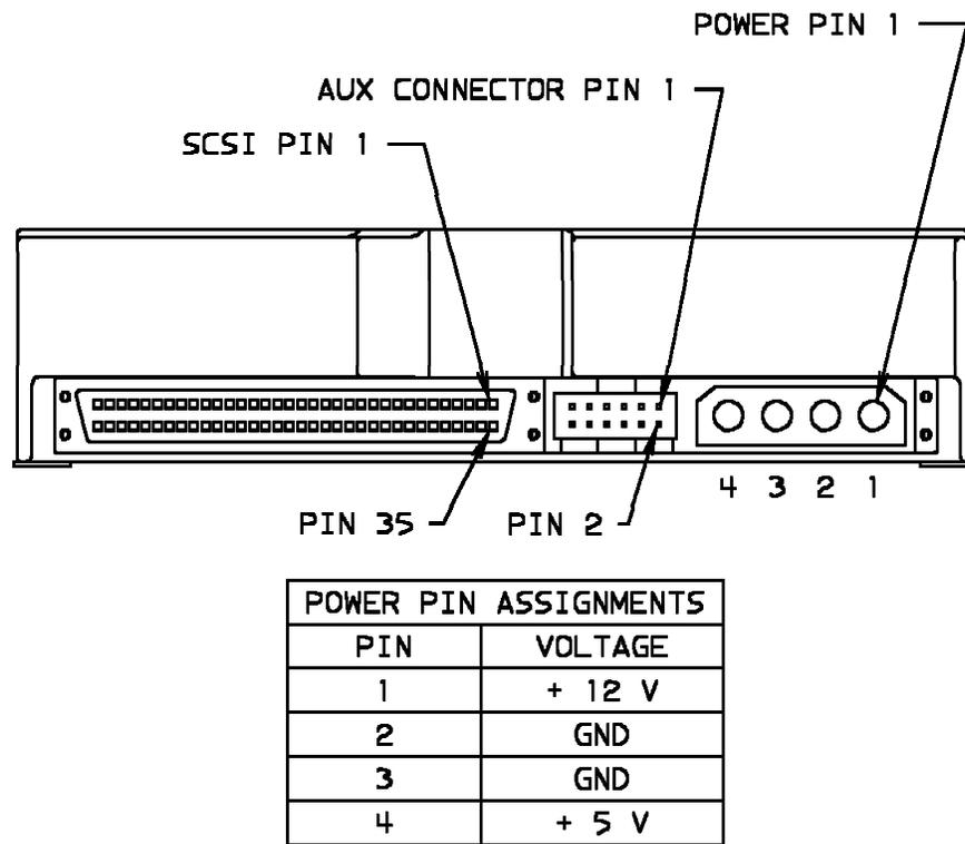
Figure 27. Electrical connectors (rear view) -- 68 pin models.
