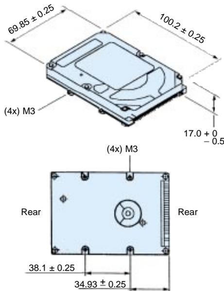
The recommended mounting screw torque is  $3 \pm 0.5$  kgf.cm.
