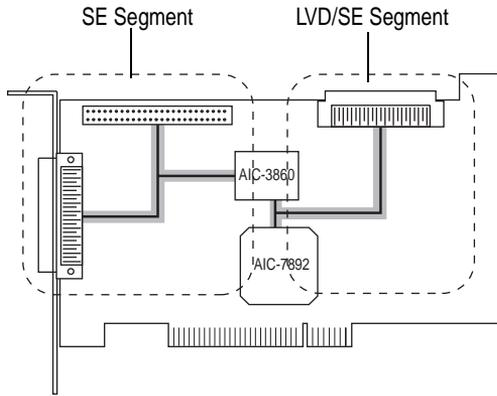
**NOTE** If you attach Wide Ultra or Ultra SCSI devices to the connector on the LVD/SE segment, the data transfer rate for *all* attached LVD SCSI devices will drop to Ultra SCSI performance levels. However, if you attach *only* LVD SCSI devices to the connector on the LVD/SE segment, data will be transferred at the maximum possible rate (80 MBytes/sec for Ultra2 devices and 160 MBytes/sec for Ultra160 devices).
