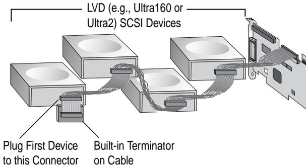
**NOTE** Internal LVD SCSI devices come from the factory with termination disabled and cannot be changed. Proper SCSI bus termination is provided by the terminator at the end of the LVD SCSI cable. See *Terminate the Ends of the SCSI Bus* on page 5 for more information.
