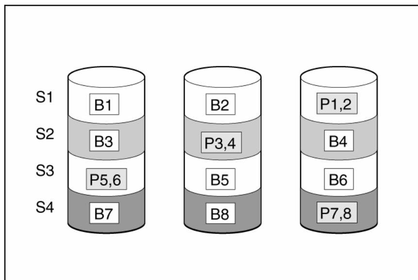
When a physical drive fails, data that was on the failed drive can be calculated from the remaining parity data and user data on the other drives in the array. This recovered data is usually written to an online spare in a process called a **rebuild**.
