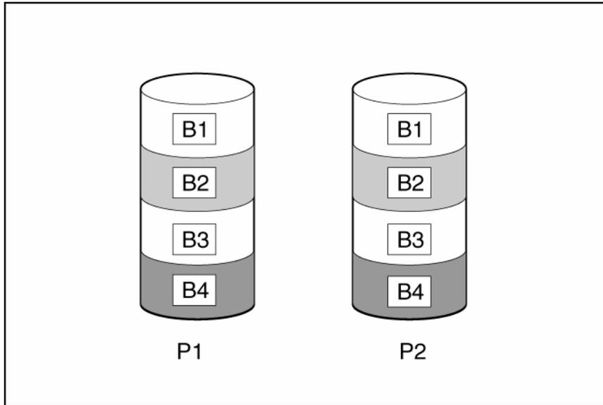
When the array has more than two physical drives, drives are mirrored in pairs.
