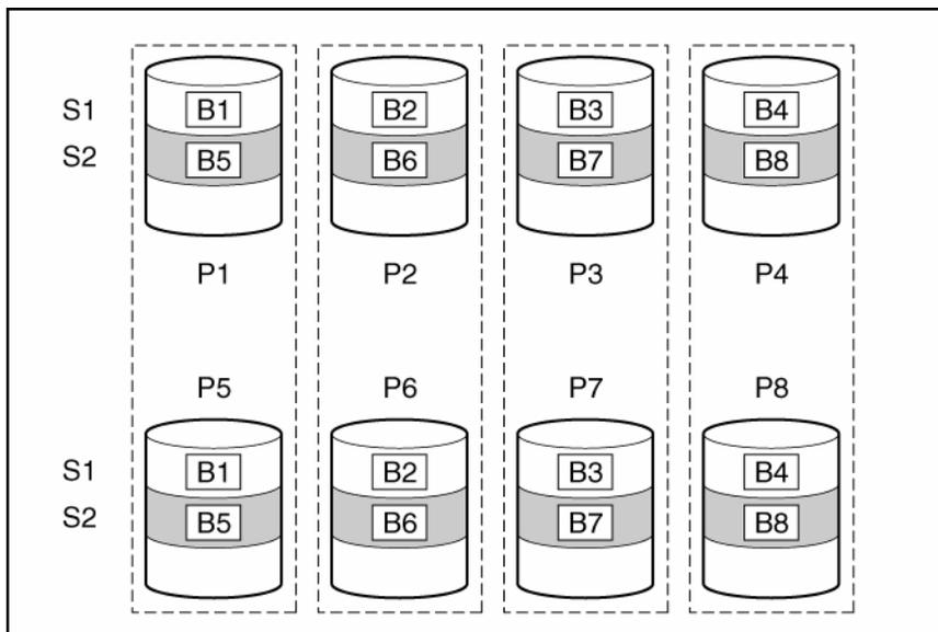
In each mirrored pair, the physical drive that is not busy answering other requests answers any read requests that are sent to the array. (This behavior is called **load balancing**.) If a physical drive fails, the remaining drive in the mirrored pair can still provide all the necessary data. Several drives in the array can fail without incurring data loss, as long as no two failed drives belong to the same mirrored pair.
