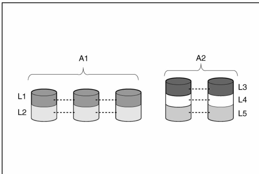
Each logical drive in an array is distributed across all of the physical drives within the array. A logical drive can also extend across more than one port on the same controller, but it cannot extend across more than one controller.
