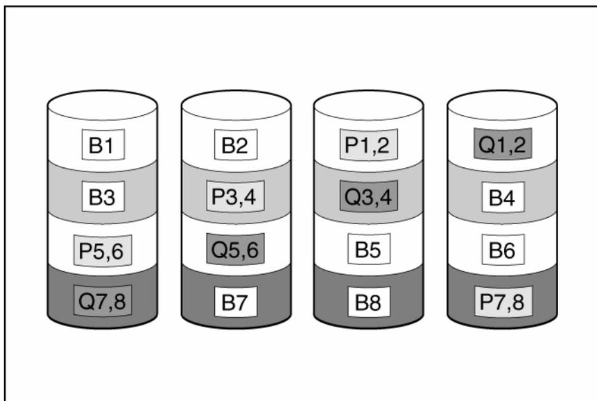
This method is most useful when data loss is unacceptable but cost is also an important factor. The probability that data loss will occur when an array is configured with RAID 6 (ADG) is less than it would be if it was configured with RAID 5.
