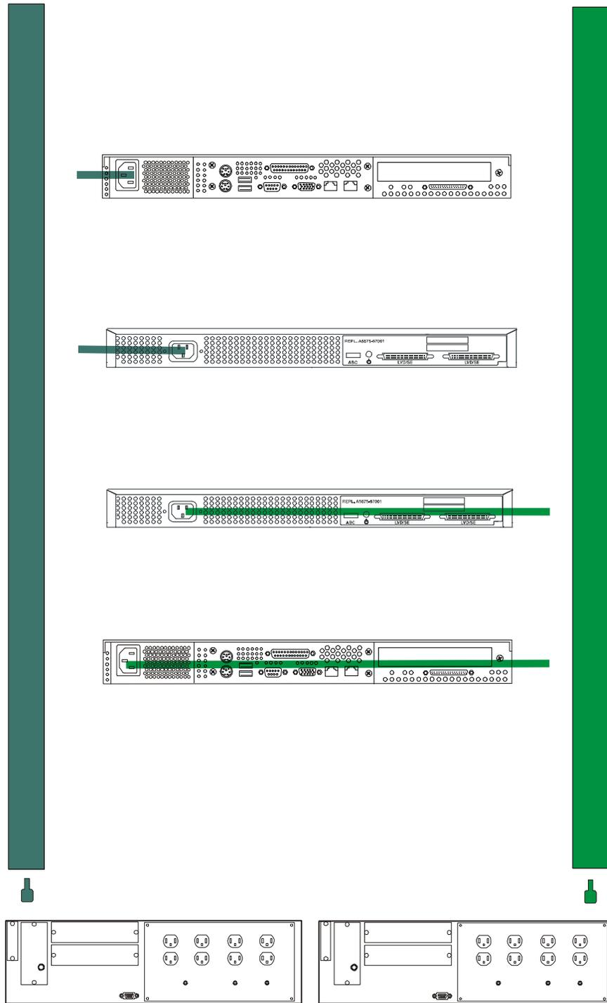
**Power Cabling to Separate Power Circuits**
