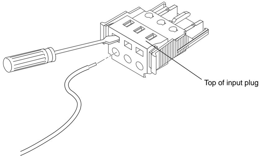
**FIGURE 2-10** Opening the Cage Clamp Using a Screwdriver
