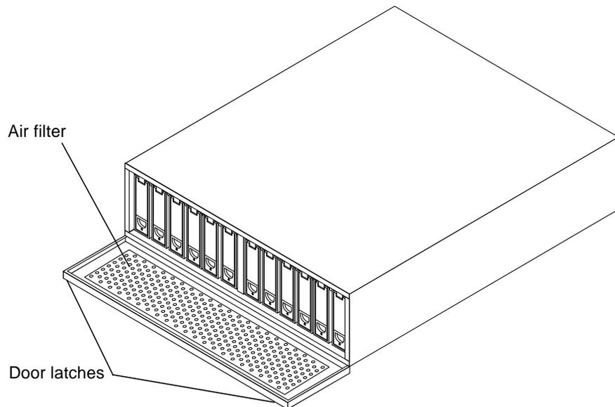
FIGURE 4-5 Removing and Replacing the Air Filter
