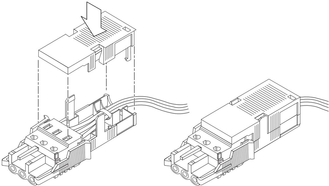
**FIGURE 2-15** Assembling the Strain Relief Housing
