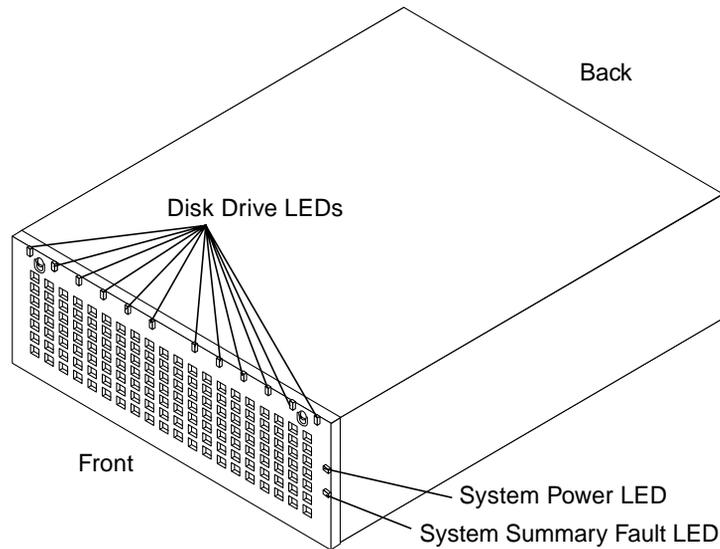
**FIGURE 6-1** Locating the Front Panel LEDs (Netra st A1000 System)
