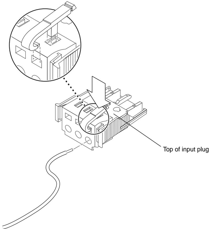
**FIGURE 2-9** Opening the DC Input Plug Cage Clamp Using the Cage Clamp Operating Lever
