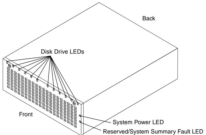
**FIGURE 6-3** Locating the Front LEDs (Netra st D1000 System)
