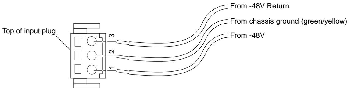
**FIGURE 2-11** Assembling the DC Input Power Cable
