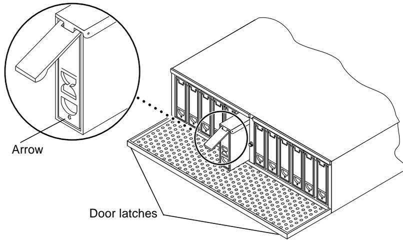
FIGURE 5-1 Adding or Replacing a Disk Drive
