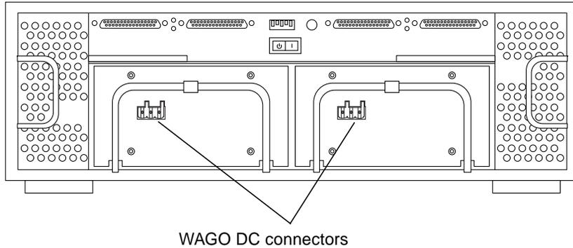
**FIGURE 1-13** Neutra st D1000 Rear View (DC Version with WAGO DC Connectors)
