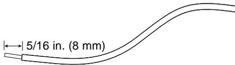
**FIGURE 2-4** Striping the Insulation from the Cable
