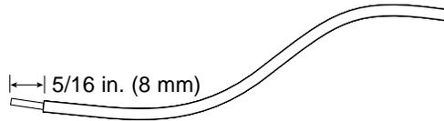
**FIGURE 2-8** Stripping the Insulation From the Wire
