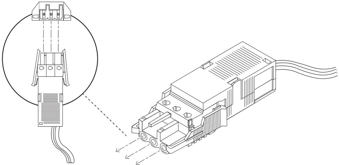
**FIGURE 3-15** Connecting the DC Input Power Cable to the *WAGO* DC Connector
