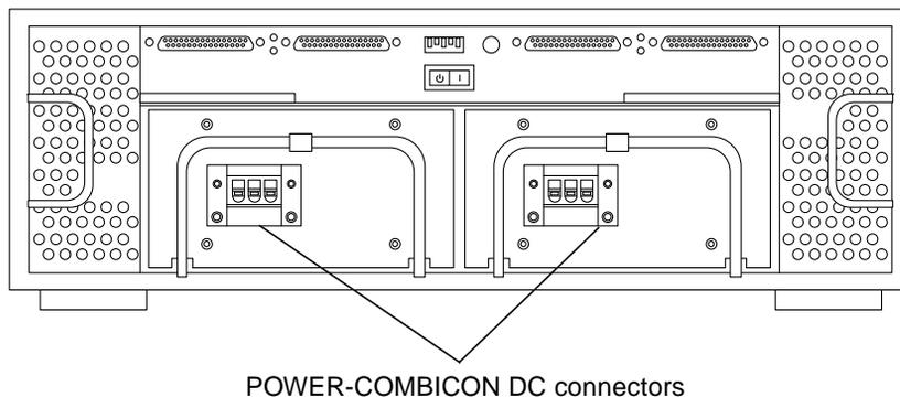
**FIGURE 1-12** Netra st D1000 Rear View (DC Version with POWER-COMBICON DC Connectors)
