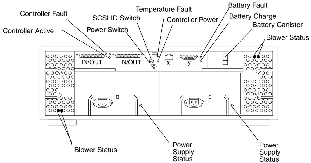
**Figure 8.** Sun StorEdge A1000 array rear view
