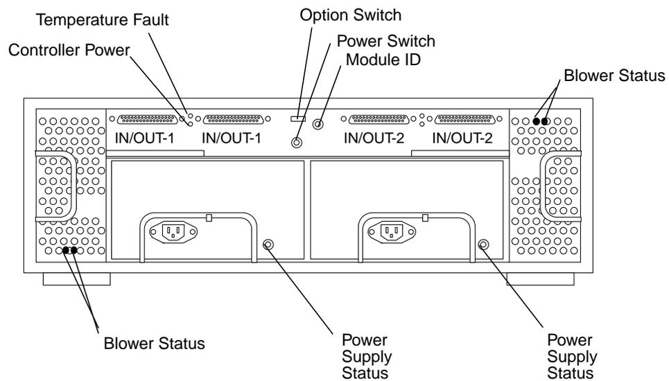
**Figure 9.** Sun StorEdge D1000 array rear view
