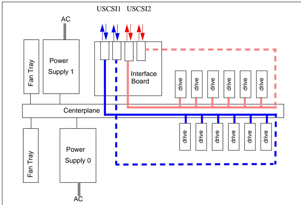
Figure 4. Sun StorEdge D1000 array system architecture
