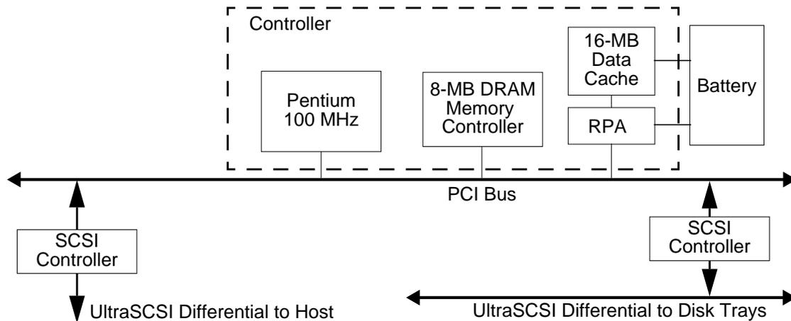
Figure 5. Sun StorEdge A1000 array controller board architecture
