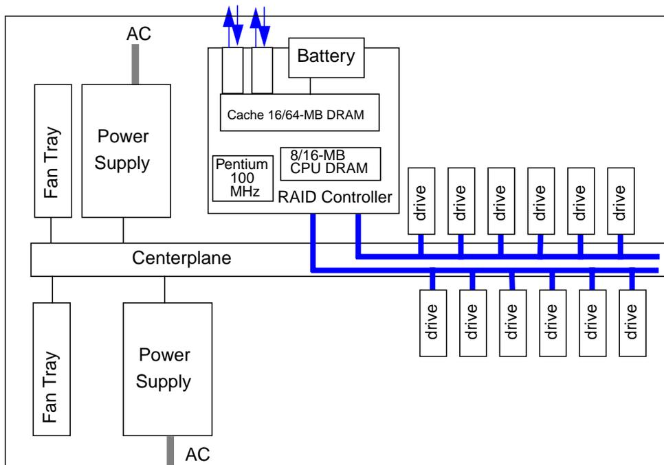
Figure 3. Sun StorEdge A1000 array system architecture
