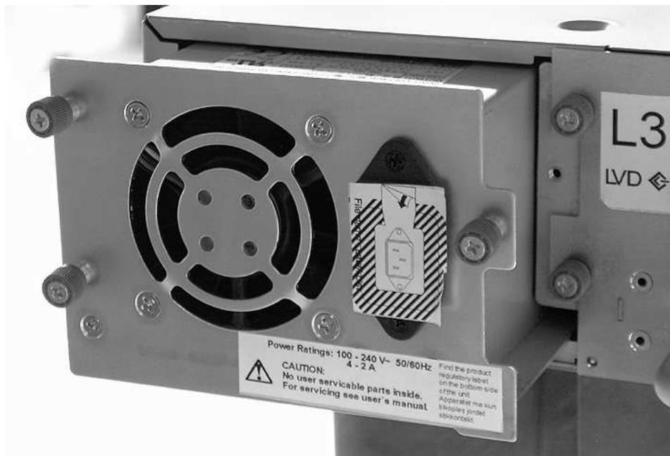
Figure 145. A power supply being removed from a 2U library
