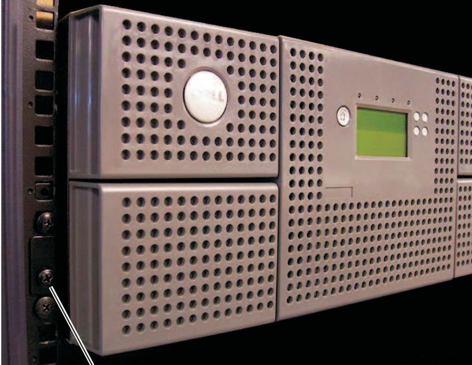
Figure 147. Removing the two mounting bracket screws anchoring the library to the rack (one screw on each side of the library)
