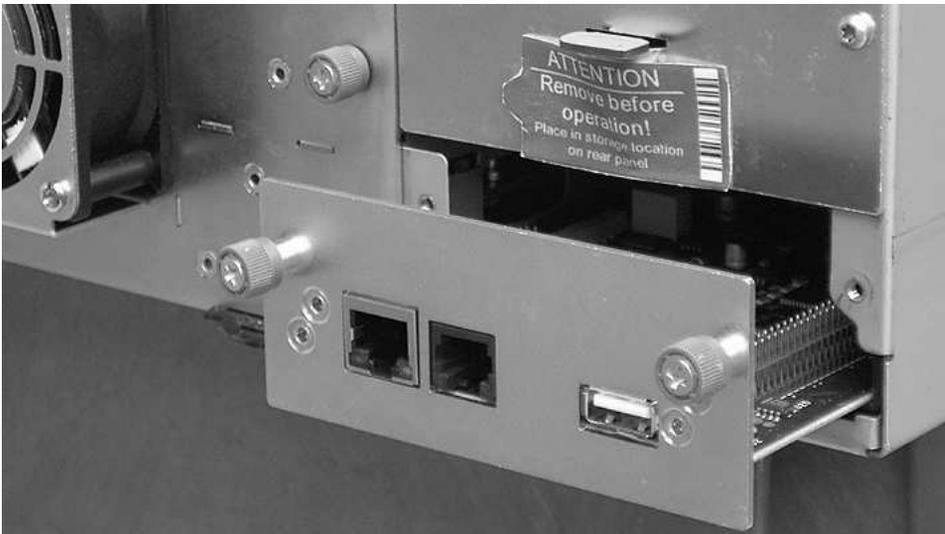
Figure 154. Removing a Library Controller Card from the library
