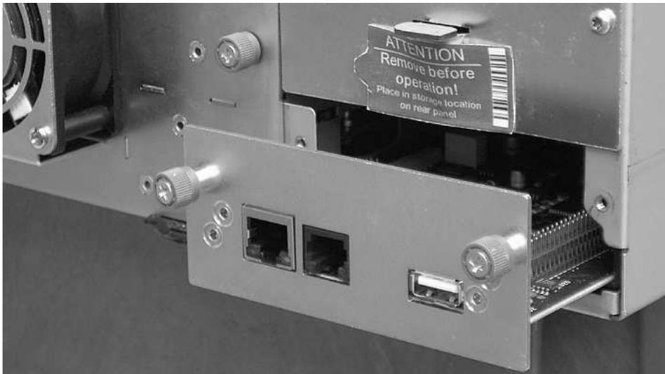
Figure 146. A Library Controller Card being removed from the library
