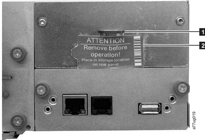
Figure 137. Shipping Lock and Label Storage Location
