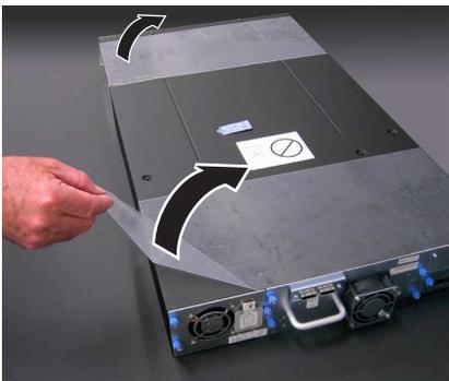
Figure 19. Removing the plastic protective sheets from the library
