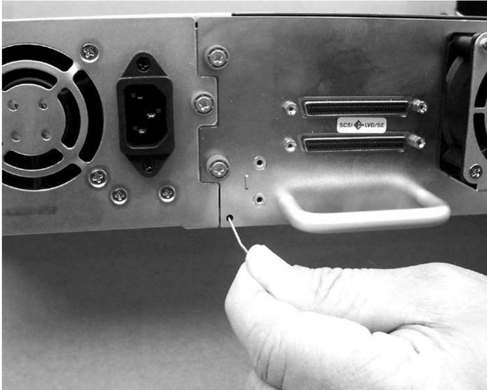
Figure 132. Access holes for the left magazine
