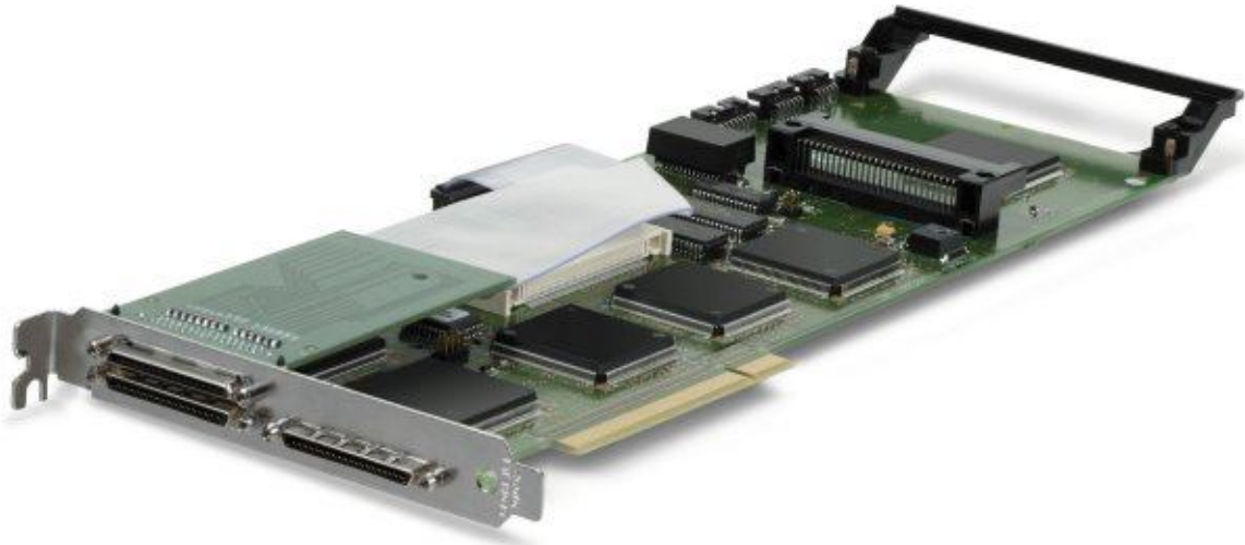
Figure 3. ServeRAID II adapter with third channel cable
