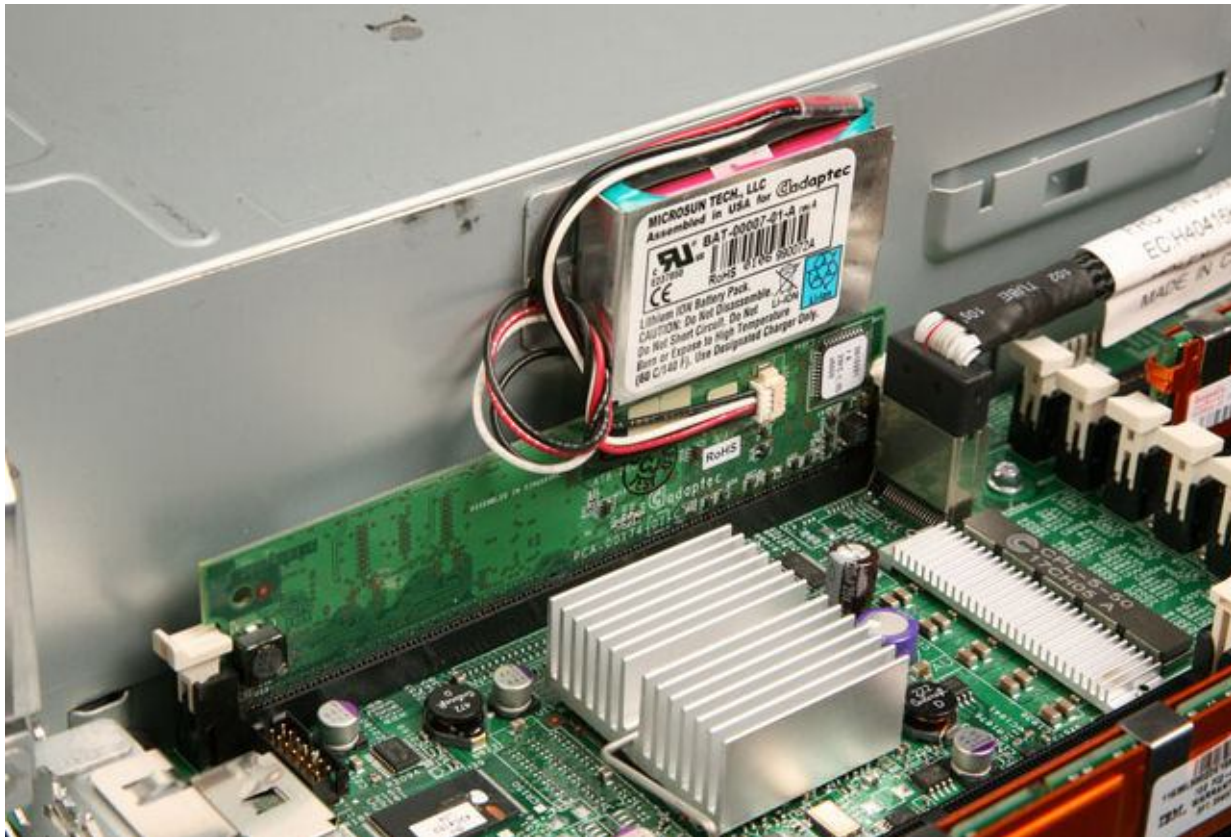
Figure 20. ServeRAID 8k installed in an x3650
