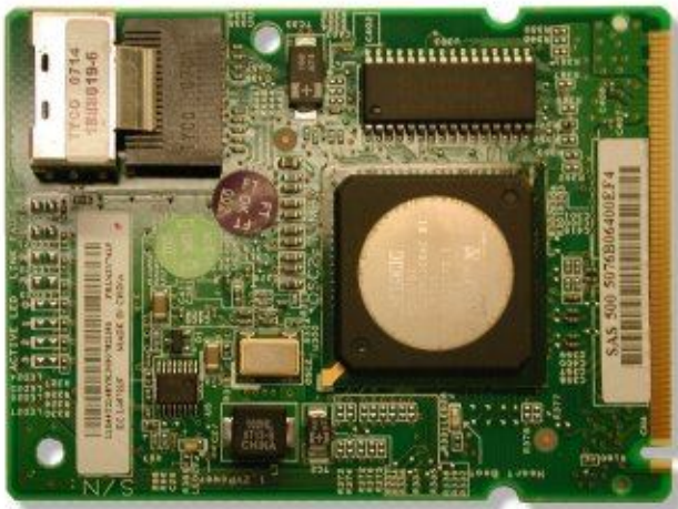
Figure 25. IBM ServeRAID-BR10il SAS/SATA PCIe Controller
