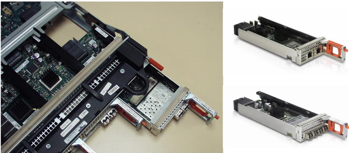
**Figure 1. CX4 UltraFlex I/O module addition and iSCSI and Fibre Channel I/O Modules**
