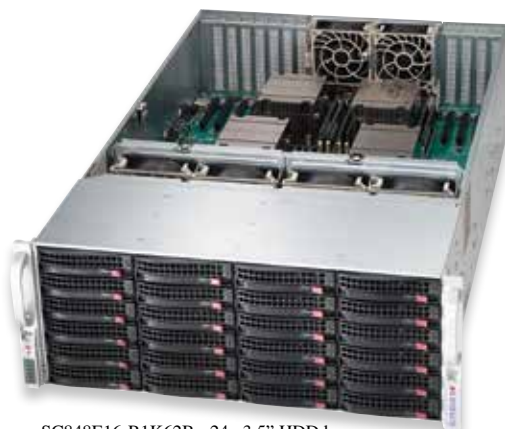
SC848E16-R1K62B - 24x 3.5" HDD bays
