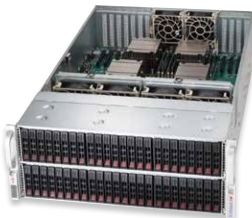
SC418E16-R1K62B2 - 48x 2.5" HDD bays
