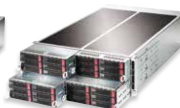
SYS-F628R3-R+ Series 4-Node, Rear I/O, 16 DIMMs 6x SAS/SATA3 + 2 NVMe drives per node
