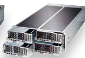
SYS-F628R2-F+ Series (shown) SYS-F628R3-F+ Series 4 DP Nodes, Front I/O, 16 DIMMs
