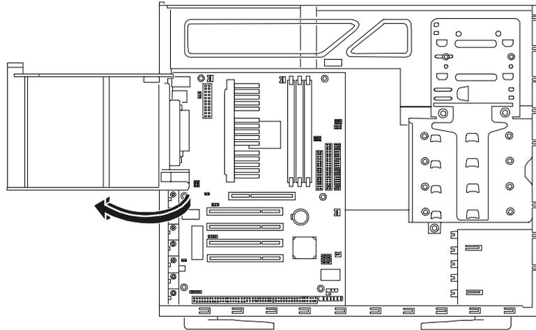
**Figure 4-1. Moving the Air Duct**
