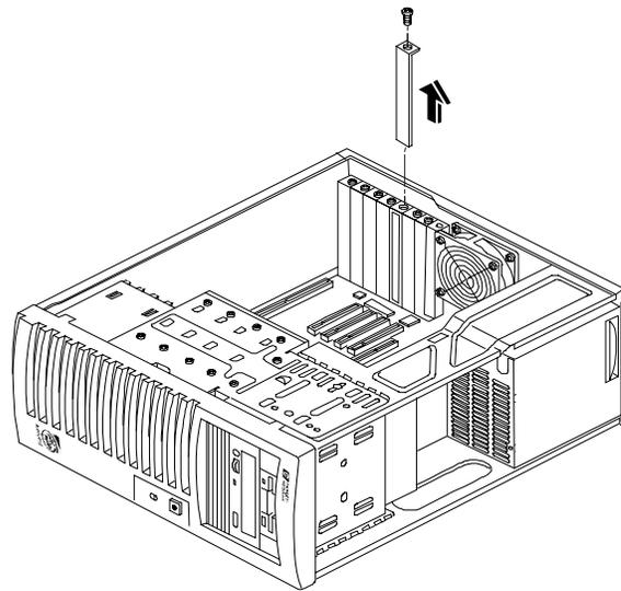
**Figure 6-2. Removing the Accessory Slot Cover**
