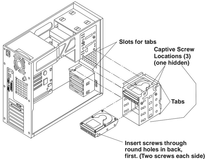
**Figure 4-3. Adding a Hard Disk Drive**
