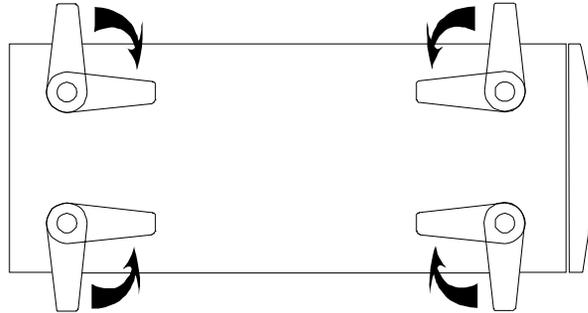
**Figure 3-4. Turn Feet Inward before Laying the NetServer on Its Side**
