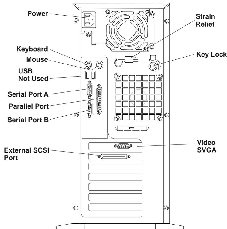
Figure 2-3. Rear Panel and Ports
