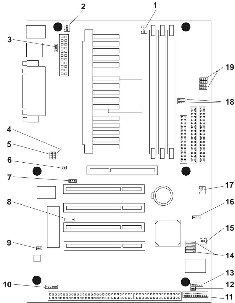
Figure A-2. Jumper and Connector Locations
