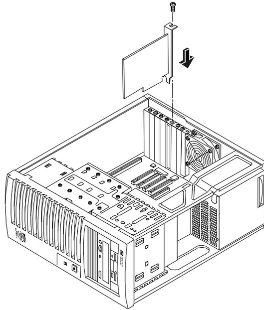
**Figure 6-3. Inserting an Accessory Board**
