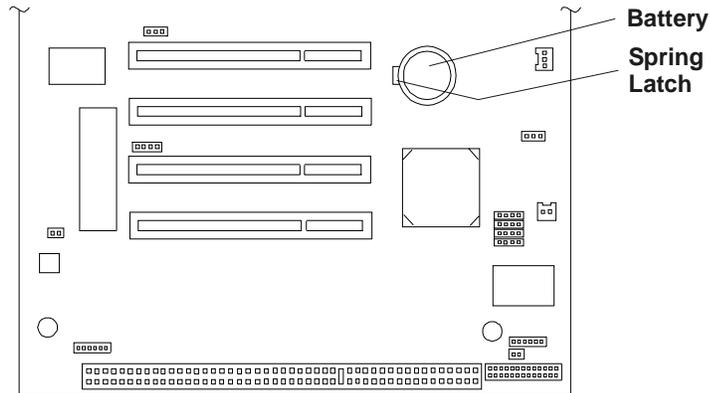
**Figure 9-2. Battery on System Board**
