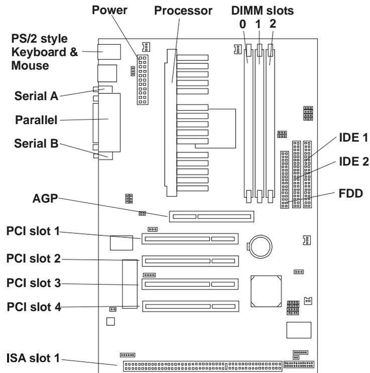
Figure A-1. HP NetServer E 200 System Board
