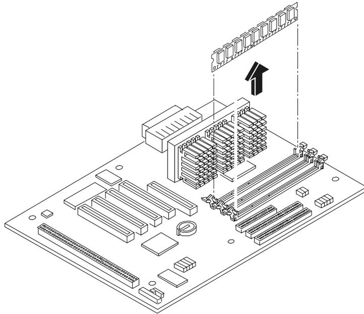
**Figure 5-3. Removing the DIMM**
