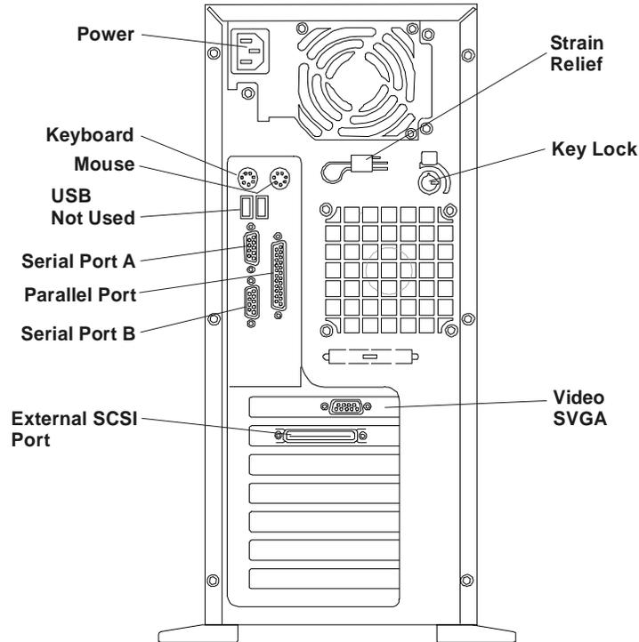
**Figure 7-1. Rear Panel Ports**
