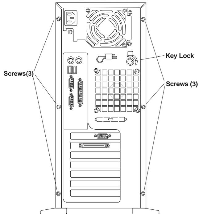
**Figure 3-1. Screws and Lock Holding on Cover**
