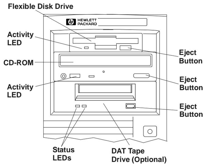
Figure 2-2. Input and Storage Device Controls and Indicators
