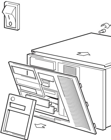
**Figure 5c: preparing mounting bay in a typical IBM server**
