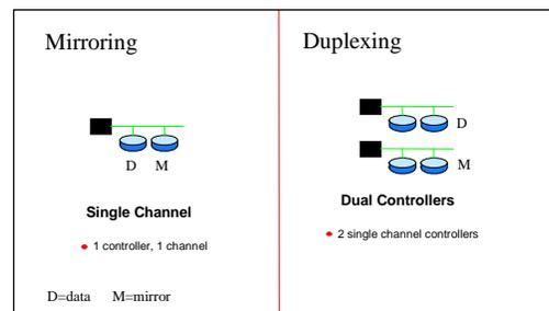
**Figure 3. SCSI Channel Configurations**
