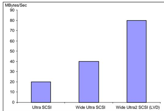
**Figure 2. Storage Controller Maximum Transfer Rate**
