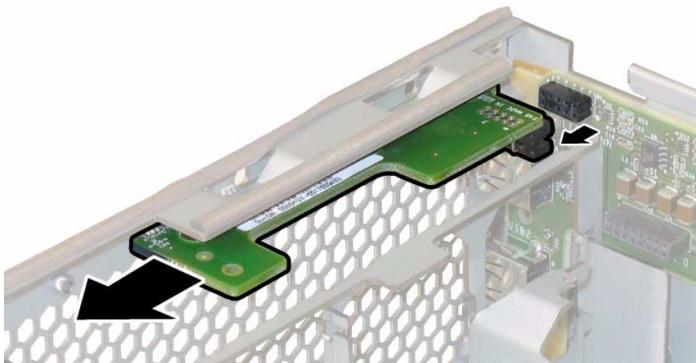
8. Remove the front panel indicator board from the chassis.
