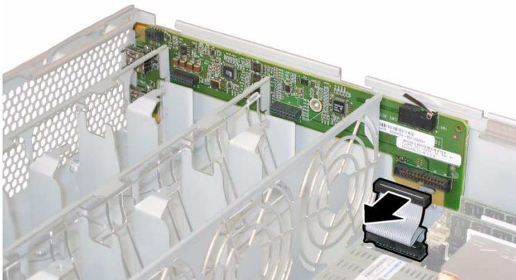
13. Unfasten the screw that secures the front I/O board to the chassis. See [FIGURE 3-39](#) or [FIGURE 3-40](#).
