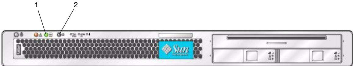
**FIGURE 2-2** Front Panel of Sun Fire X4200/X4200 M2 Server
