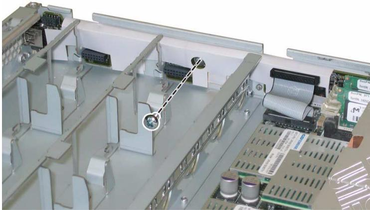
**FIGURE 3-40** Unfastening the Front I/O Board Screw From the Chassis (Sun Fire X4200 Server Shown)
