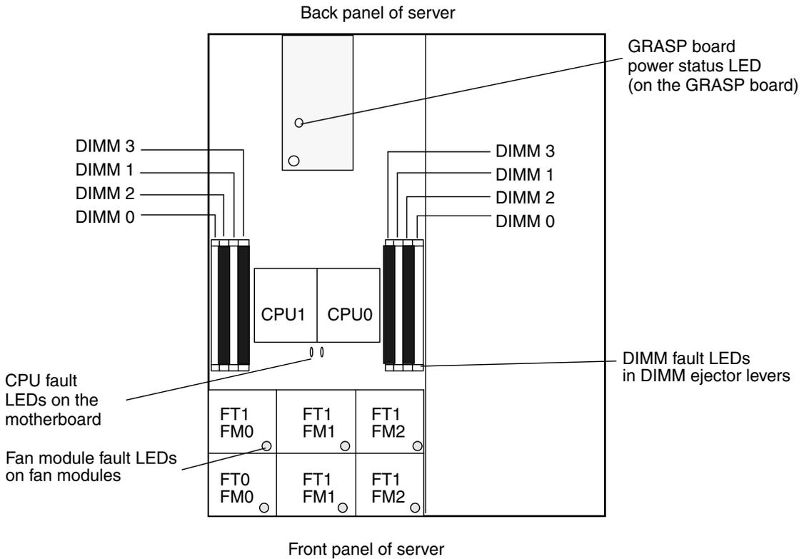
**FIGURE B-3** Sun Fire X4100/X4200 Internal LED Locations
