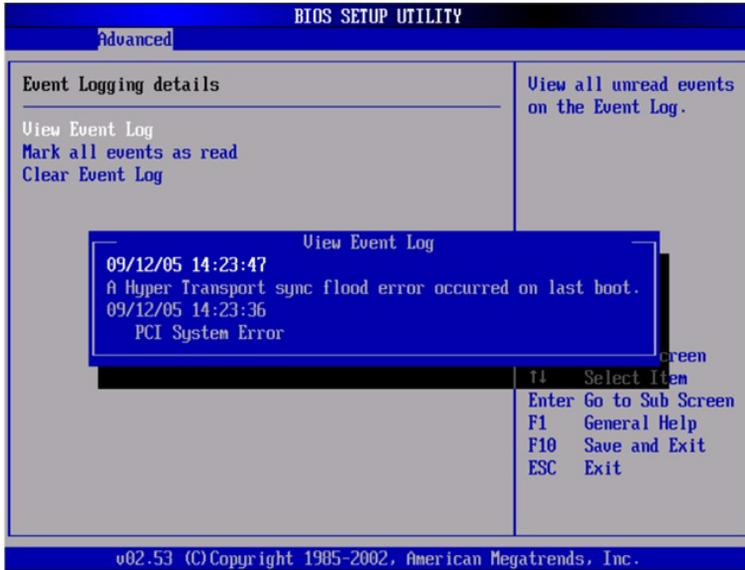
FIGURE E-6 Sample DMI Log Screen, System Error Listed
