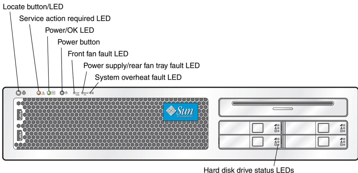
**FIGURE B-1** Sun Fire X4200/X4200 M2 Servers Front Panel LEDs
