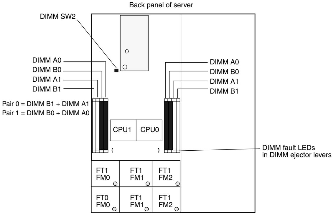
**FIGURE 1-5** Sun Fire X4100 M2/X4200 M2 DIMM Slot Locations
