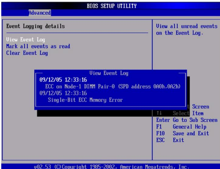
**FIGURE E-2** Sample DMI Log Screen, Correctable Error
