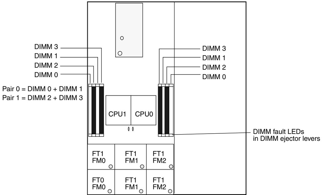
**FIGURE 1-4** Sun Fire X4100/X4200 DIMM Slot Locations
