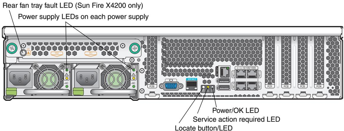
**FIGURE B-2** Sun Fire X4200/X4200 M2 Servers Back Panel LEDs
