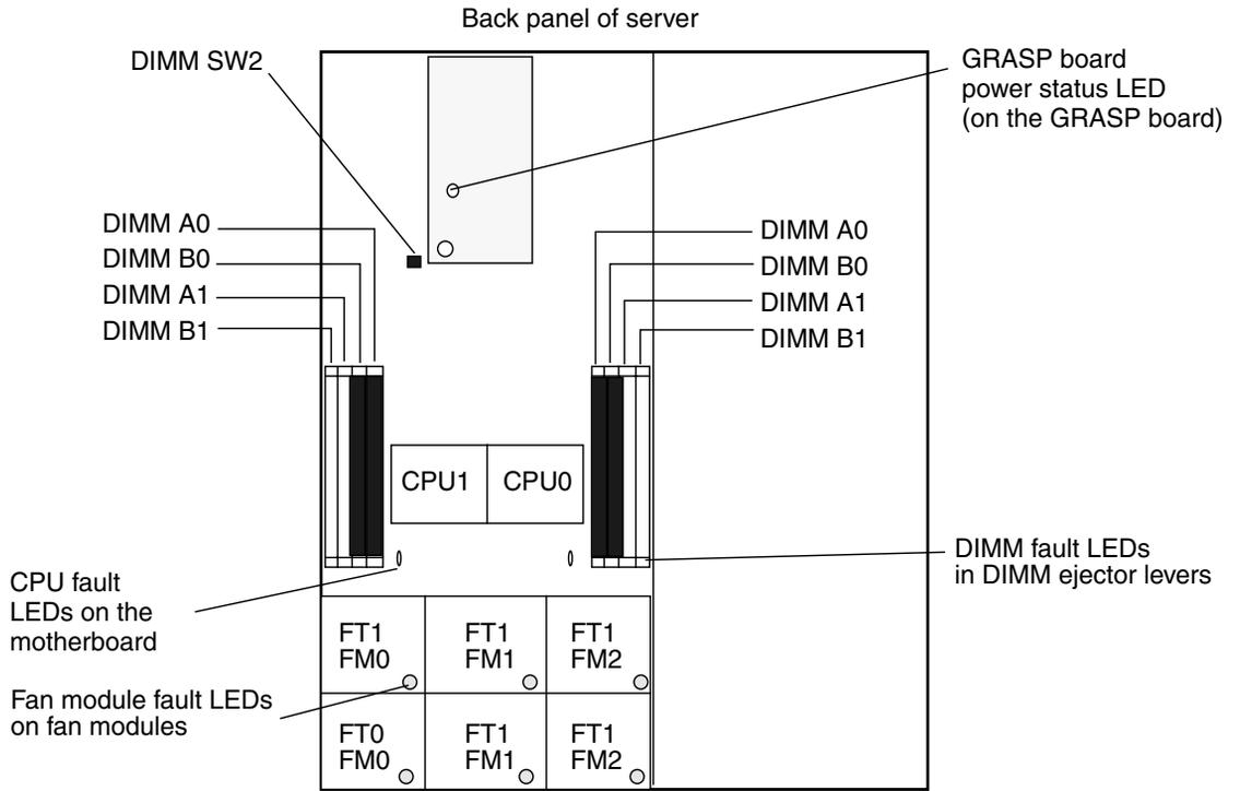
**FIGURE B-4** Sun Fire X4100 M2/X4200 M2 Internal LED Locations
