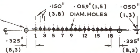
PANEL CUTOUTS VIEWED FROM UNDERSIDE (P.C. SIDE)
