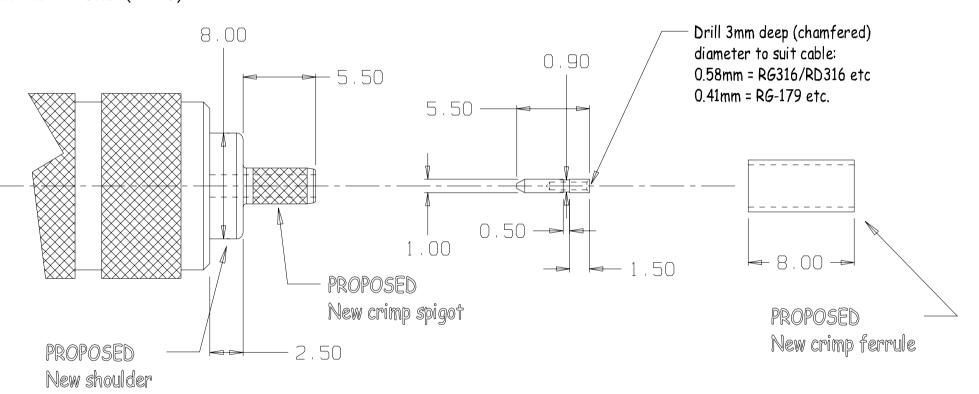
Note: This pin provides for the use of contact--registration/location finger such as is included in Suhner crimp die 76Z-0-2-1
