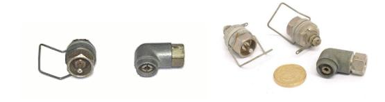
PYE connectors were developed by the Company of the same name in the 1940s and were used on many British military equipments. By modern standards, they are truly dreadful connectors, being unsealed with a totally uncontrolled characteristic impedance. Although, during WW2, they were used at frequencies up to 100MHz and perhaps even higher, it was because there was nothing else available in the UK, rather than because they were suitable for purpose.
