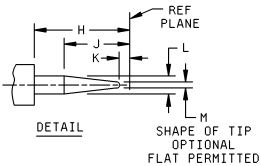
FIGURE 22. Interface, series N, pin contact.
