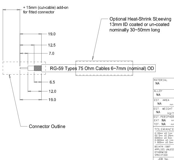
3000 CUSTOMER DRAWING Reference No. SIZE CASA Modular Systems 5 ☐ Modular Systems **A4** DESCRIPTION 11PAL-EF125RG59 A Semi-Crimp PAL Plugs & Sockets from YuBright etc. DWG. SCALE DRAWN 27/05/19 APPROVED
