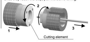
After cooling, remove the assembly from the jig. Screw the positioner B onto the assembly jig. Slide the cable into the connector until it bottoms against the positioner B. Put three rings of solder around
