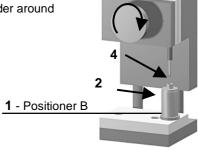
After cooling, remove the assembly from the jig. Screw dielectric recess gauge and trim dielectric.
